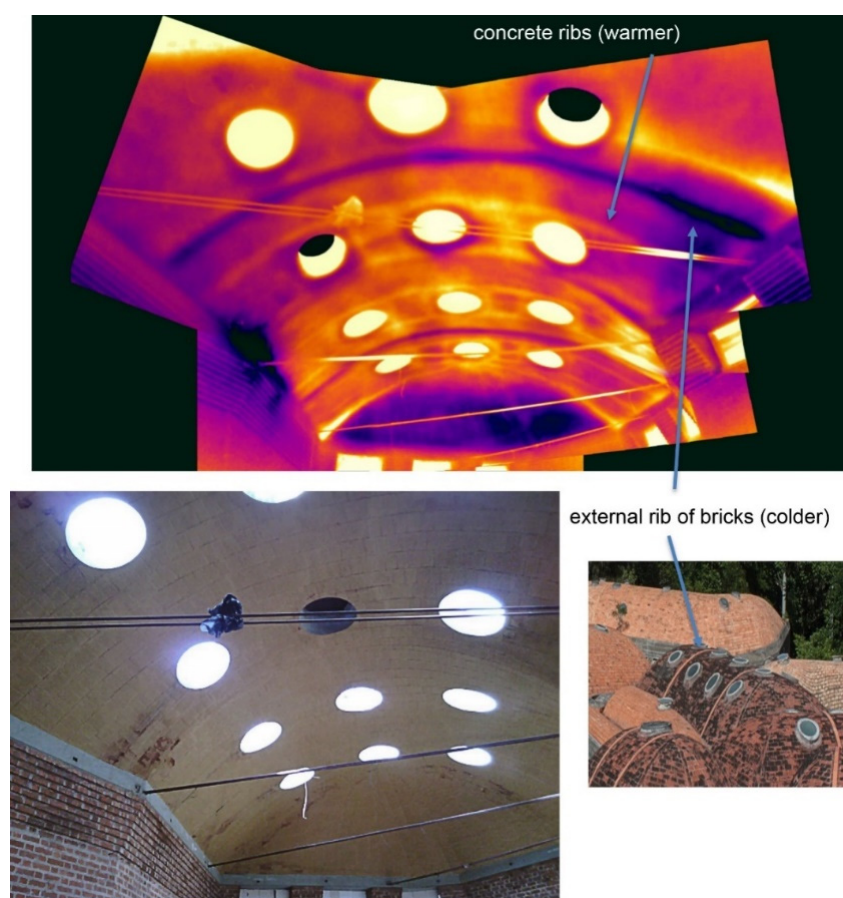
Figure 29. School of Dramatic Arts: Thermograph of a vault (thermal range 28.0–30.0 °C). 19 February 2020 at 1:00 p.m., 29.1 °C—RH 67.0% (Images by Luca Valisi).
