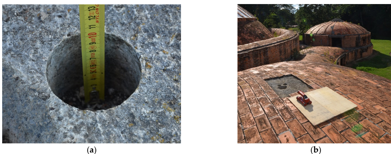
Figure 16. (a) The 10 cm hole left by previous core testing, proving the presence of a concrete slab (photos by the authors). (b) Pachometer testing performed to detect possible rebar in the same vault.
