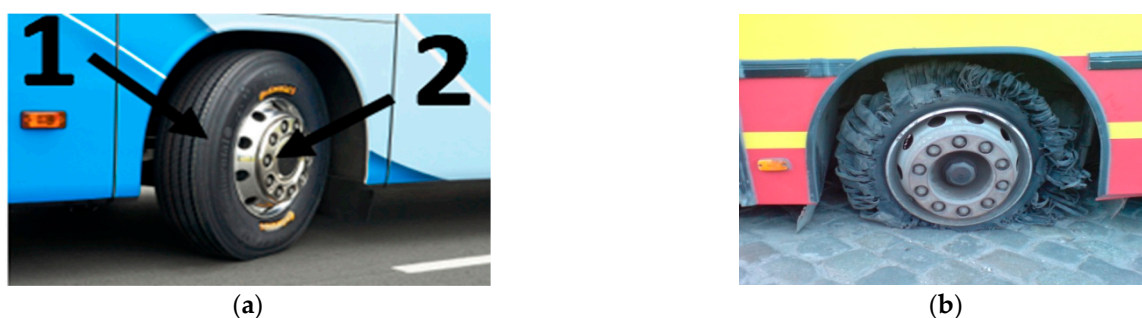
Figure 3. (a) Construction of the wheel 1—tyre, 2—rim, (b) a damaged bus tyre [22].
