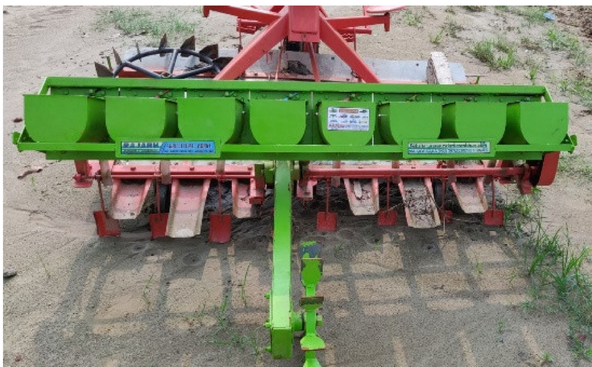
Figure 2. A self-propelled direct paddy seeder prototype with the recommended row to row (22.5 cm) and hill to hill spacing (15 cm).
