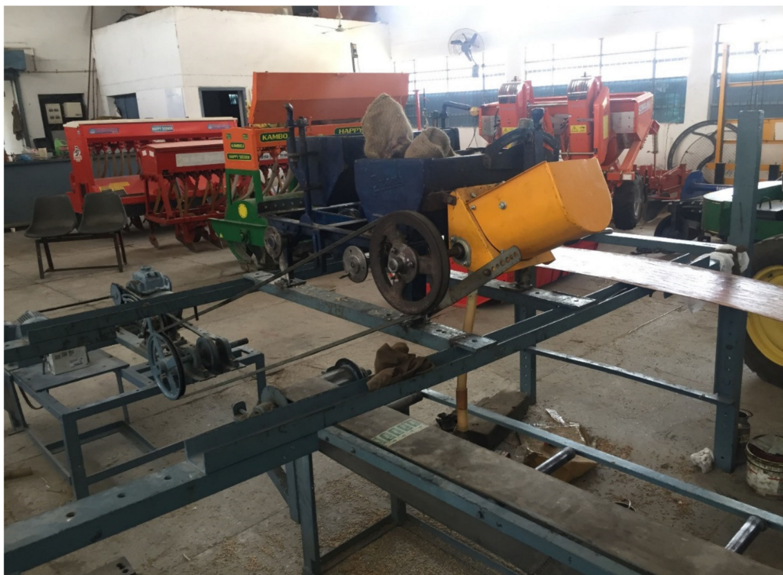
Figure 1. The test rig layout was used during the study to find the interaction between dependent and independent variables. The interaction of independent variables (different metering mechanisms, forward speeds, and pre-germination levels) was evaluated using a matrix that constituted the missing index (%), multiple index (%), and seed damage (%).
