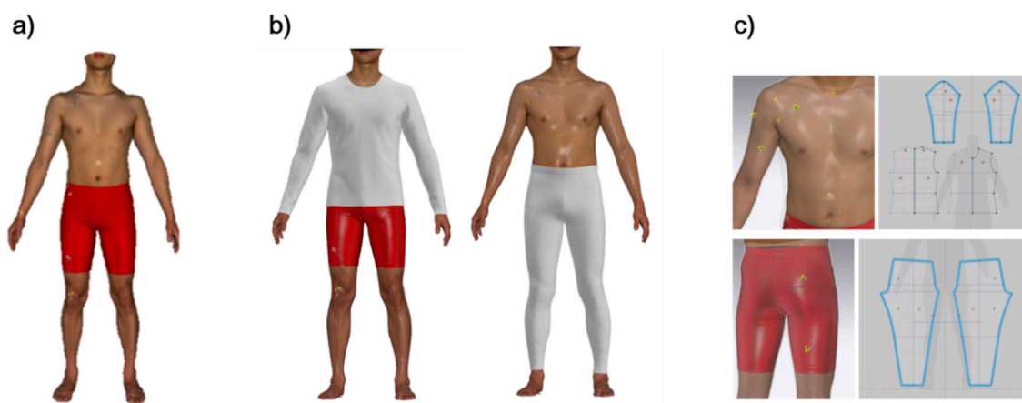
Figure 4. Preliminary process for specifying EMG electrode location: (a) a subject's scan data; (b) designing basic patterns of bodies, sleeves, and pants and its virtual fitting on scan data using CLO 3D; and (c) manual positioning EMG electrodes on the scan data on clothing patterns by adjusting transparency of the fabric.
