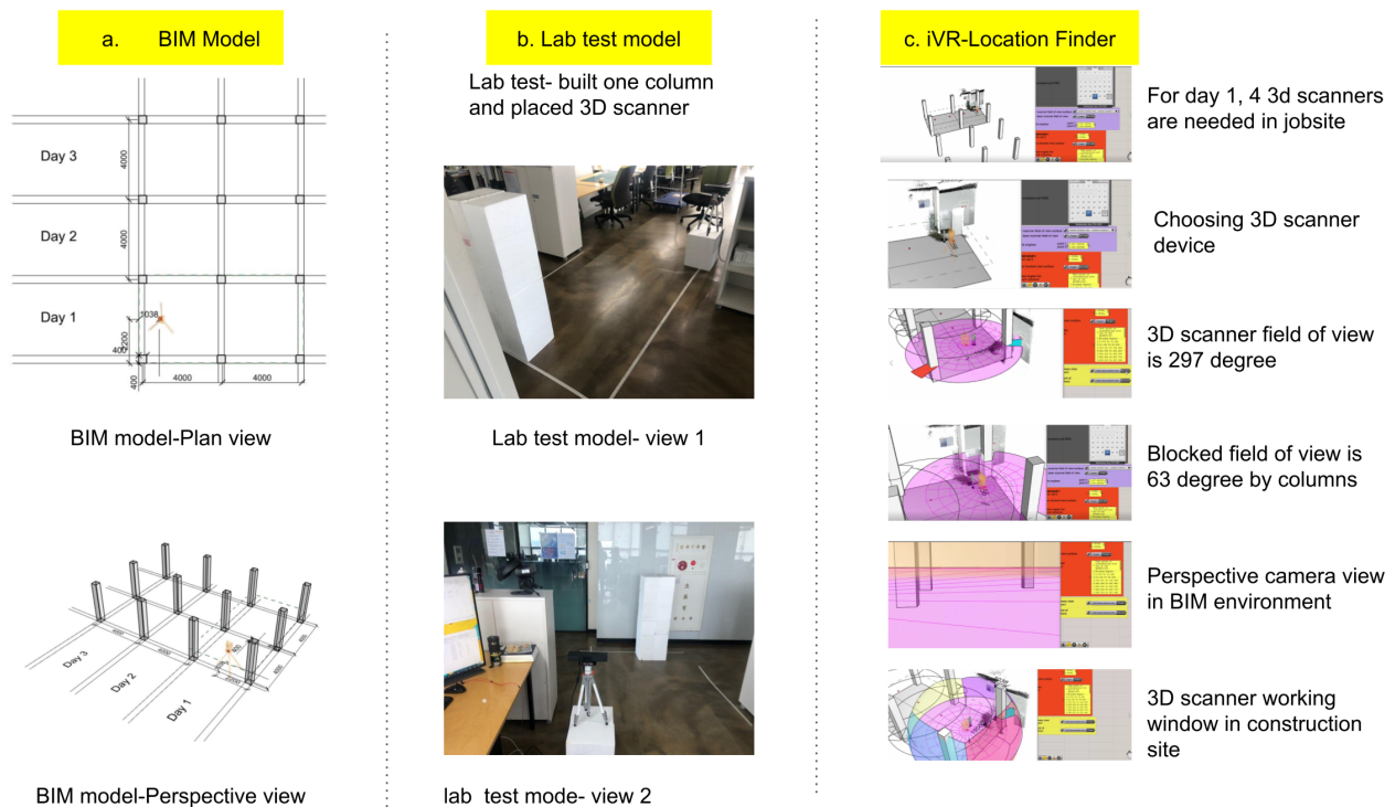
Figure 9. Case study detailed maps and 3d model + 3D scanner location: (a) virtual BIM model of column structure consist of 12 columns 4 m by 4 m span and 0.4 by 0.4 m cross-section; (b) Lab test physical model representing 3D scanner, targeted activity (one column), and building boundary lines; (c) iVR-location finder tool used to optimize 3D scanner locations in a virtual case study.
