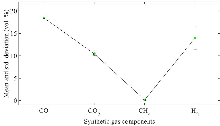
**Figure 13.** Mean and standard deviation of synthetic gas composition (vol.%) during rice husk gasification.
