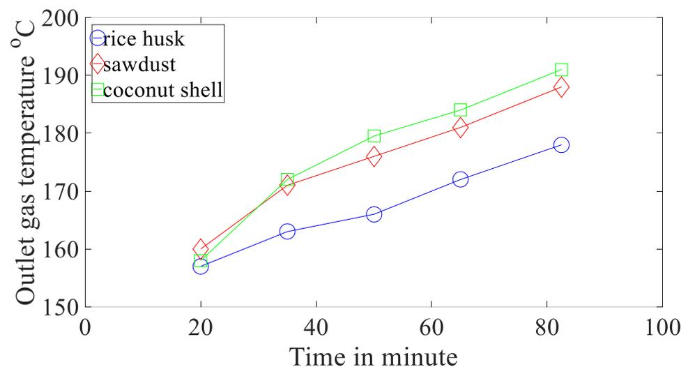
**Figure 18.** Outlet temperature of gasifier reactor for rice husk, sawdust, and coconut shell.
