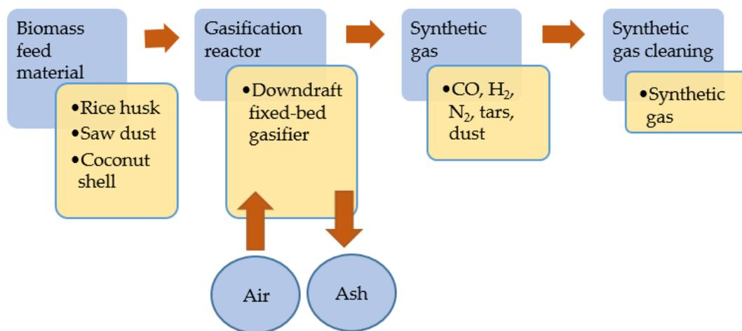
**Figure 7.** Flow diagram of the biomass gasification process.
