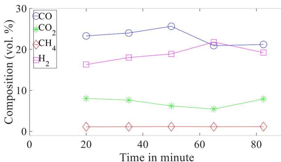
Figure 16. Synthetic gas composition in gasification of coconut shell.
