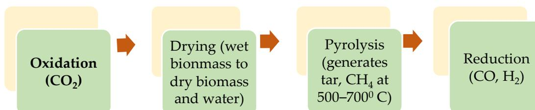
Figure 6. Biomass gasification process and reactions of gasifier.
