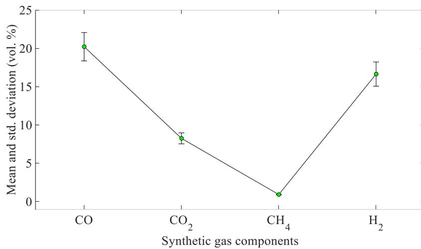
**Figure 15.** Mean and standard deviation of synthetic gas composition (vol.%) during sawdust gasification.
