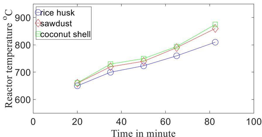
**Figure 11.** Combustion temperature during the rice husk, sawdust and coconut shell gasification process.
