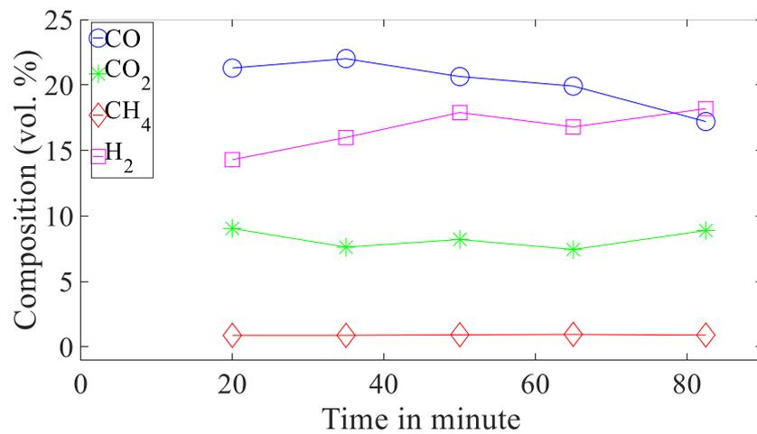
**Figure 14.** Synthetic gas composition in gasification of sawdust.
