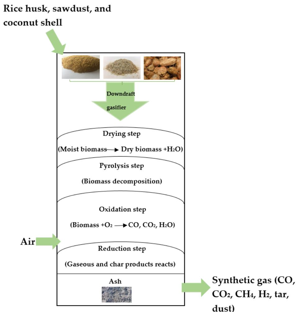
**Figure 10.** Schematic diagram of rice husk, sawdust, and coconut shell gasification.
