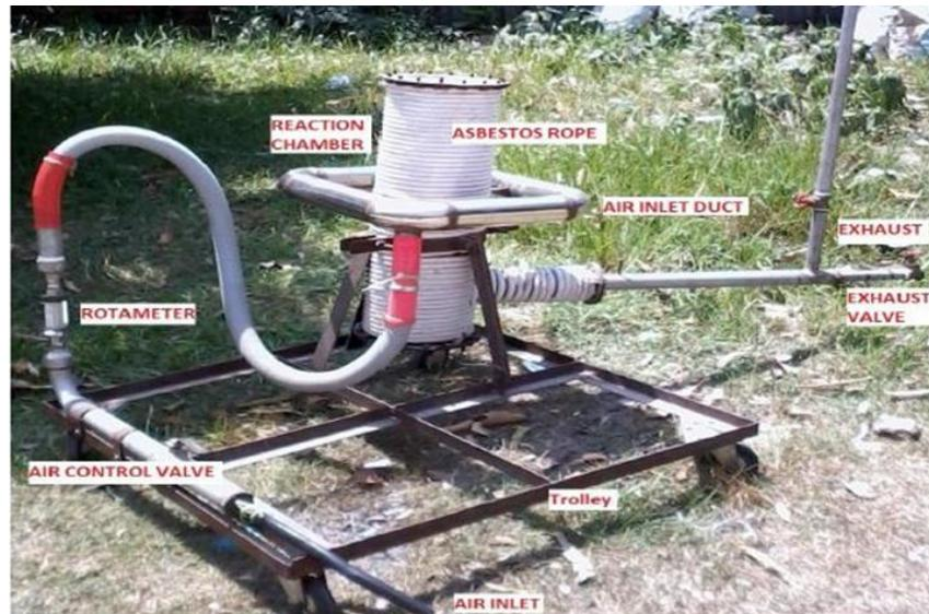
Figure 8. Photograph of the fixed-bed downdraft gasifier unit.
