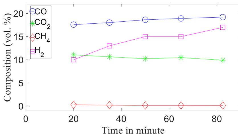
**Figure 12.** Synthetic gas composition in gasification of rice husk.
