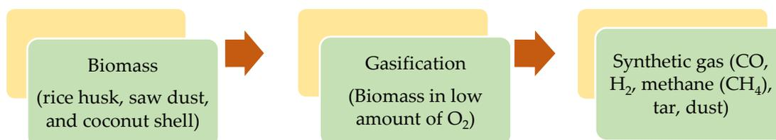
Figure 5. Flow diagram used during rice husk, sawdust, and coconut shell gasification.
