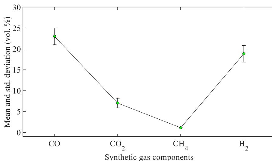
Figure 17. Mean and standard deviation of synthetic gas composition (vol.%) during coconut shell gasification.
