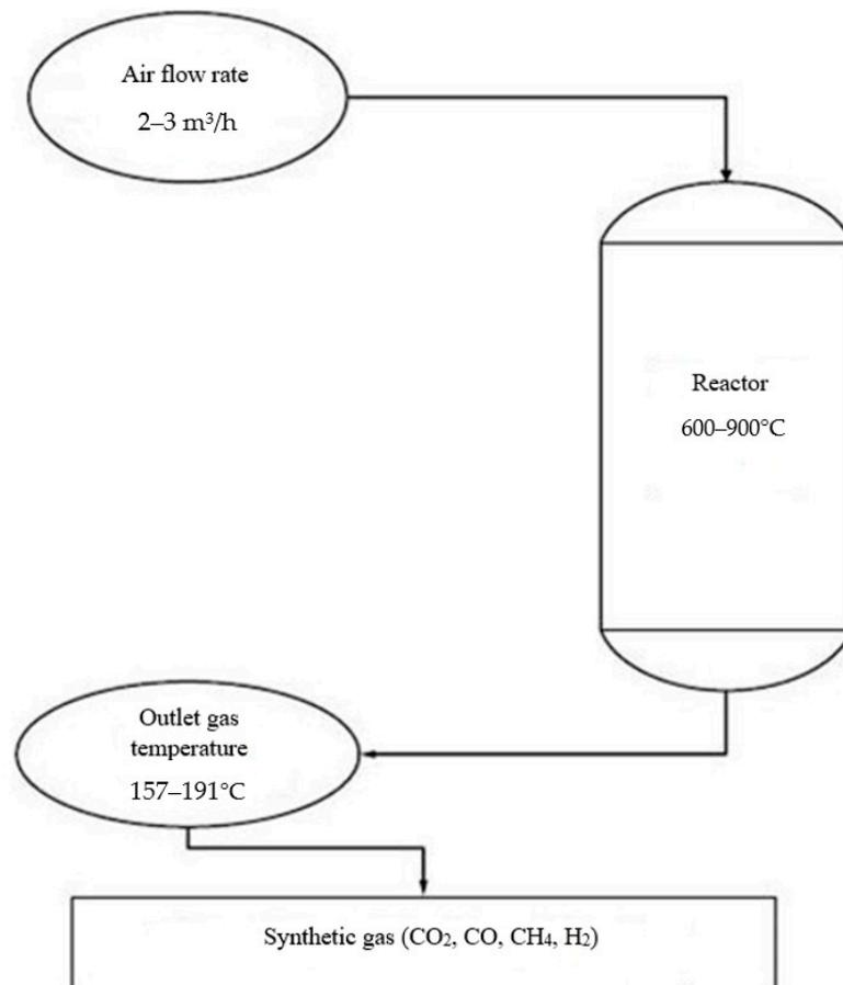
Figure 9. Flow Diagram of the fixed-bed downdraft gasifier unit.
