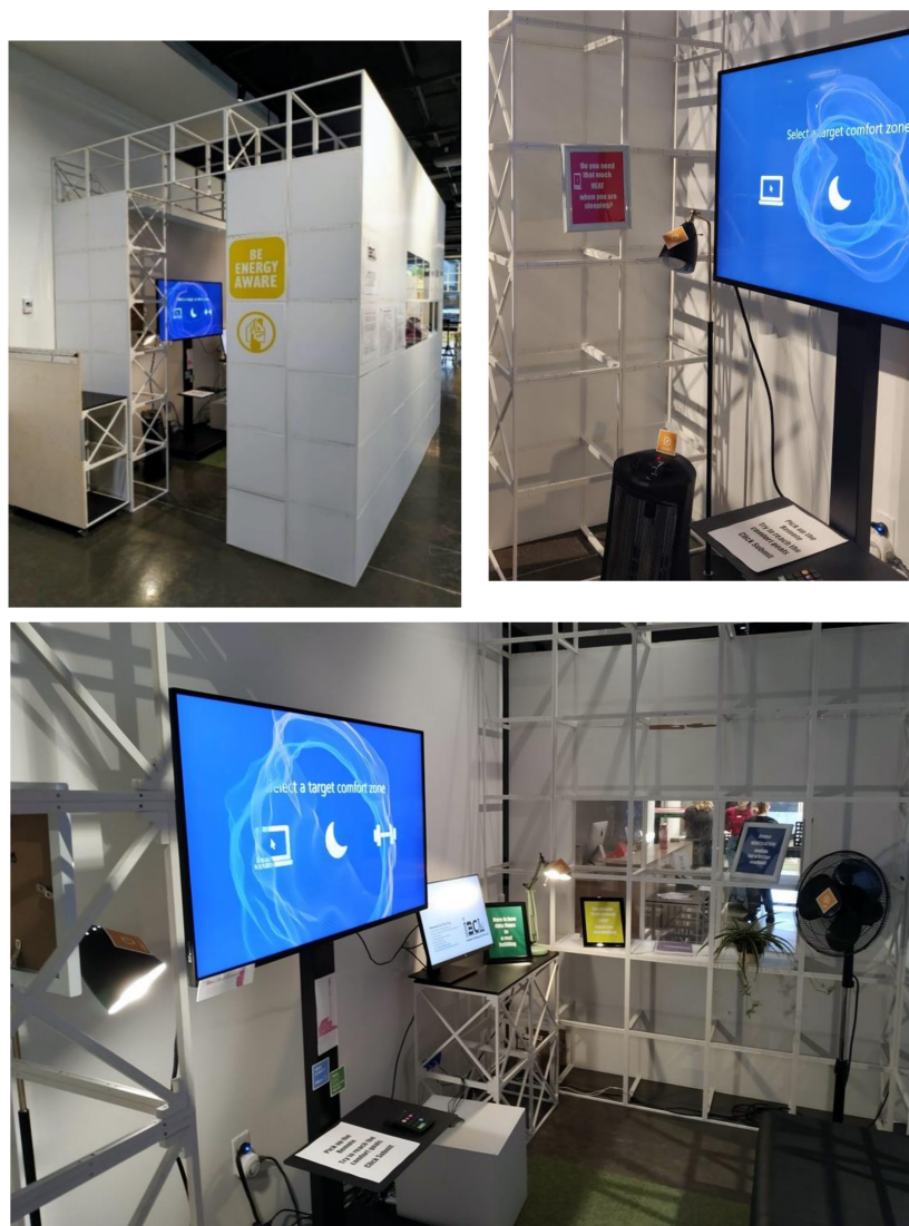
Figure 1. Test room setup fitted with a heater, fan, and two lighting units, the comfortable leather couch and plants, and the interactive control interface.
