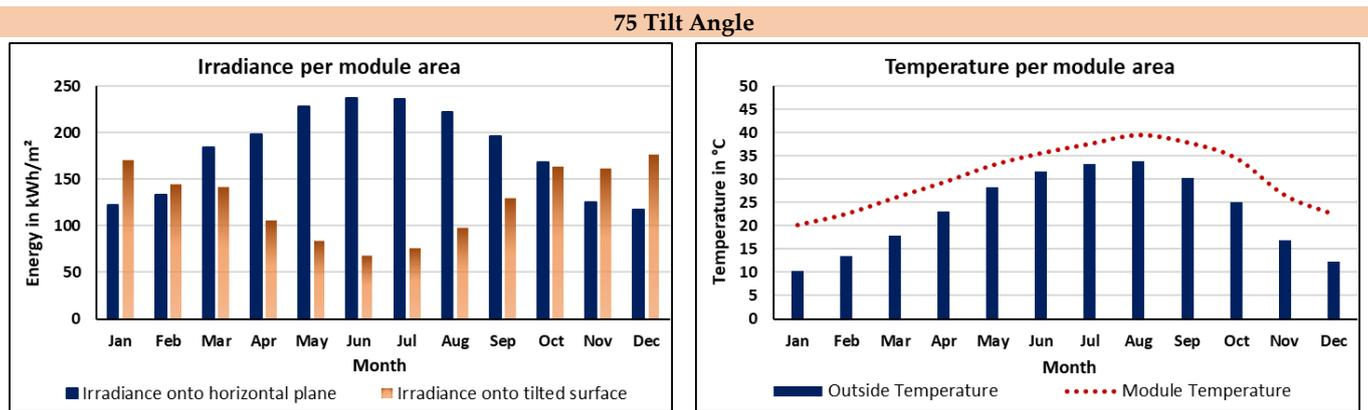
**Figure 9.** The relationship between the irradiance and the temperature of the PV module.
