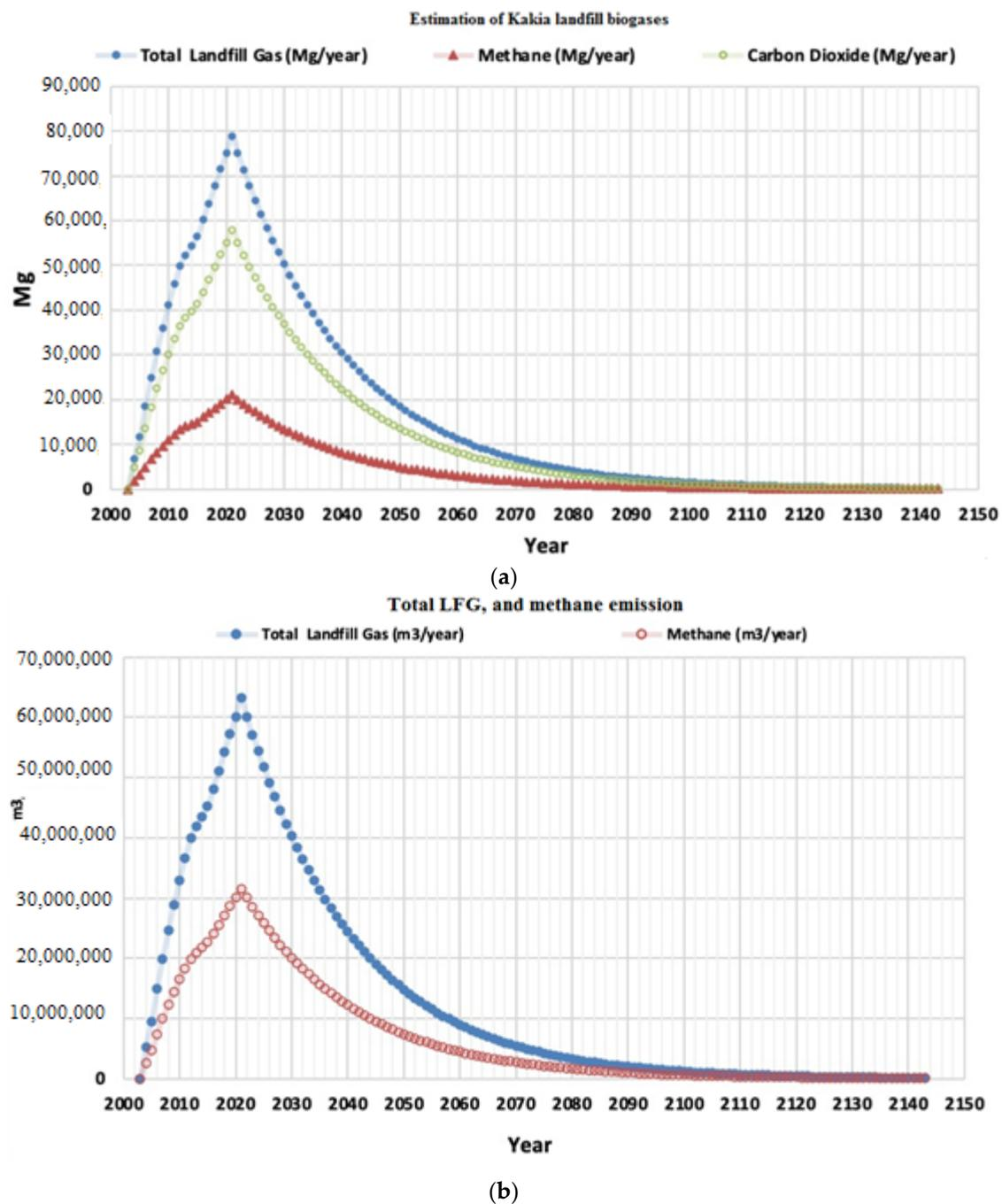
**Figure 5.** (a) Landfill gas emission estimation in Mg/year, (b) total LFG, and methane emission estimation in  $\text{m}^3/\text{year}$  for Kakia landfill utilizing the LandGEM model for the years 2003–2143.
