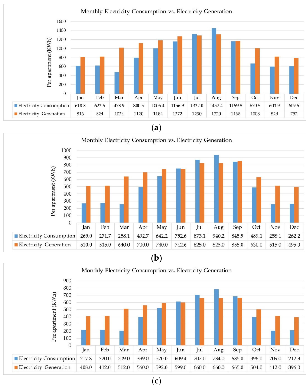
Figure 10. Comparison between monthly electricity consumption of the base case and generation electricity by PV cells. (a) Reference building 7, (b) reference building 8, (c) reference building 9.
