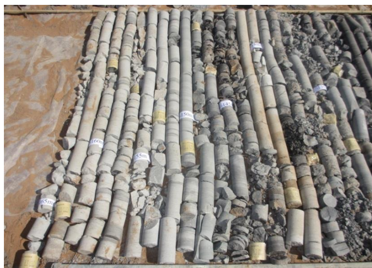
Figure 15. Fracture characteristics of cores in the hole depth of 135–166 m.
