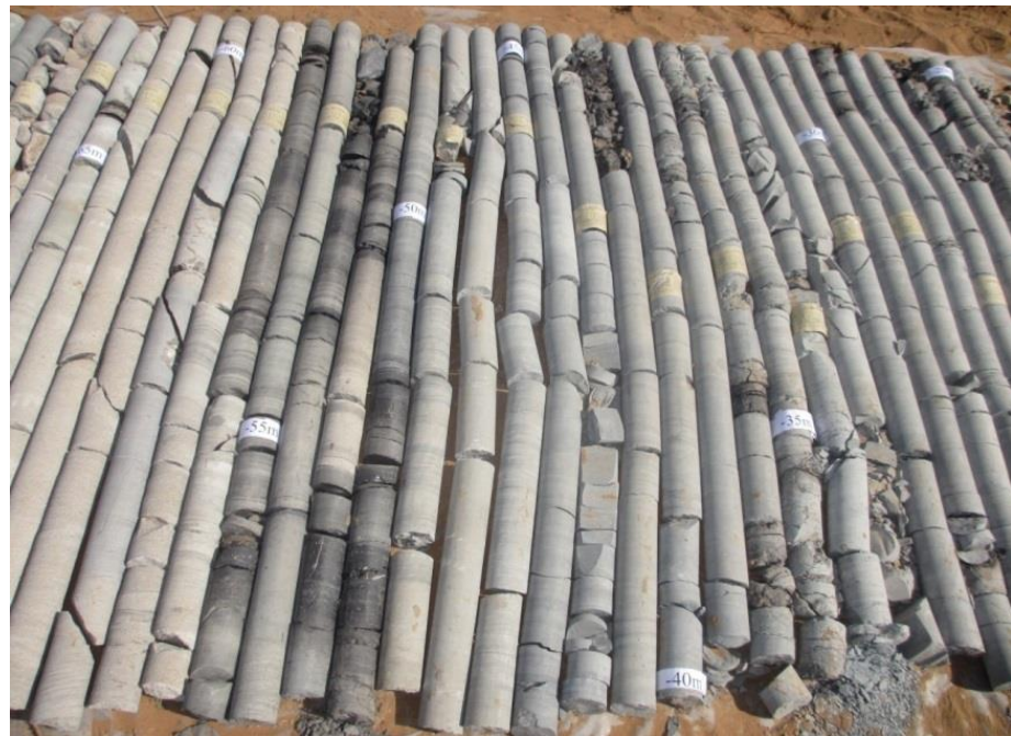
Figure 17. Fracture characteristics of cores in the hole depth of 30–65 m.
