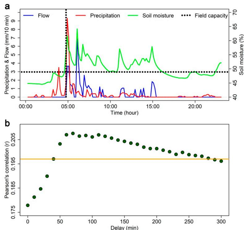
**Figure 3.** (a) Selection of a typical event hydrograph for TB-48 (14 May 2019). (b) Correlogram between precipitation and drainage time series for TB-48 (from 16 September 2019 to 13 February 2020).
