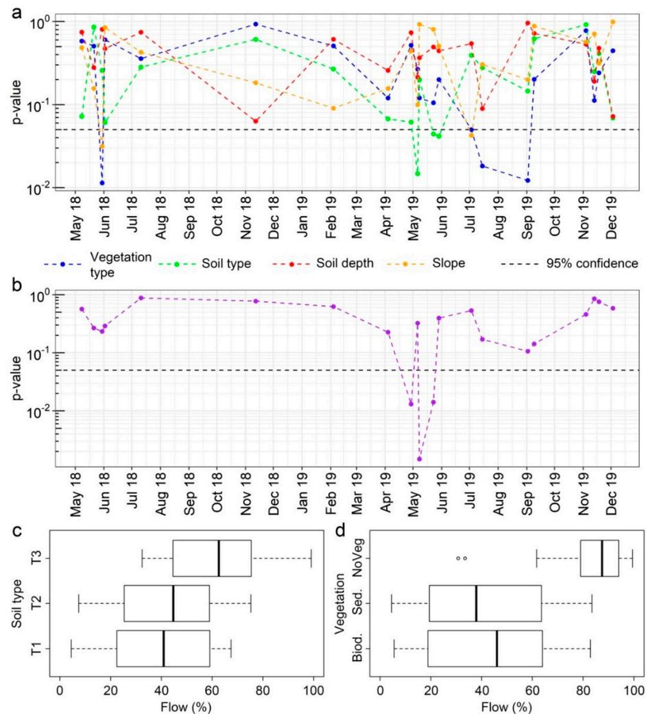
**Figure 2.** (a) Results of the multiway analysis of variance (ANOVA) on the tested factors vs. the drainage flow for 48 TBs. (b) Results of the fertilization process on 12 TBs. Finally, box plots representing differences in drainage flow for (c) soil and (d) vegetation type (Sed. = *Sedum*; Biod. = biodiverse; NoVeg = bare soil).
