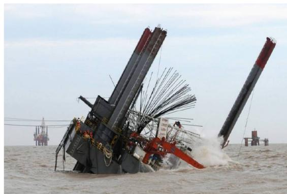
**Figure 2.** ShengLi Well Workover Platform III overturning accident [3].
