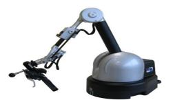
Figure 4. Haptic feedback device Virtuose 6D TAO.
