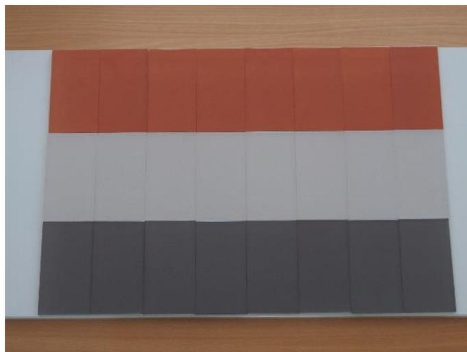
**Figure 1.** Photograph of the inkjet-printed test specimen, in the colours, terracotta, grey, and anthracite (**top to bottom**), before exposure to corrosive media or radiation.
