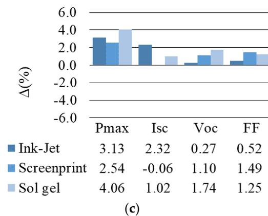
**Figure 8.** Variations in the electrical parameters of the test modules after weathering tests: DH 1000 h (a), TC 200 cycles (b) and DH 200 h plus UV 60 kWh/m<sup>2</sup> (c).
