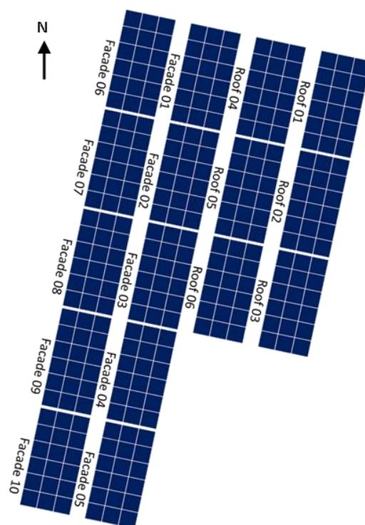
**Figure 12.** BIPV test site, module layout for test site (roof and façade).
