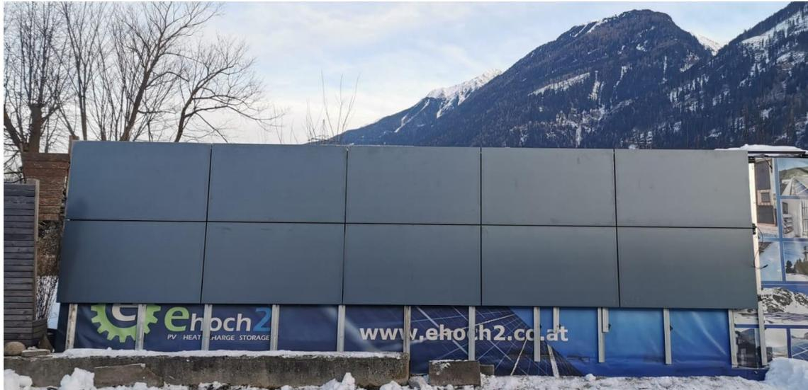
Figure 3. Photo of the test façade with grey screen-printed modules.
