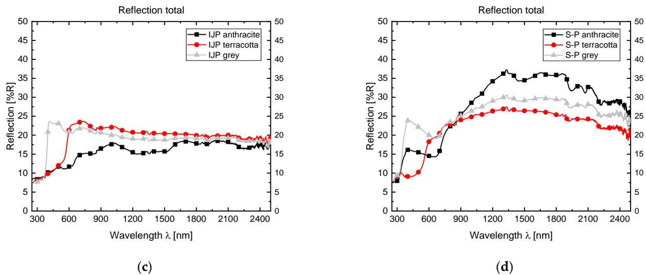
**Figure 4.** Total hemispherical reflection of uncoated glass (a), terracotta-, grey-, and anthracite-coloured glasses, coated by sol-gel technology (b), inkjet printing (c), and screen-printing (d).
