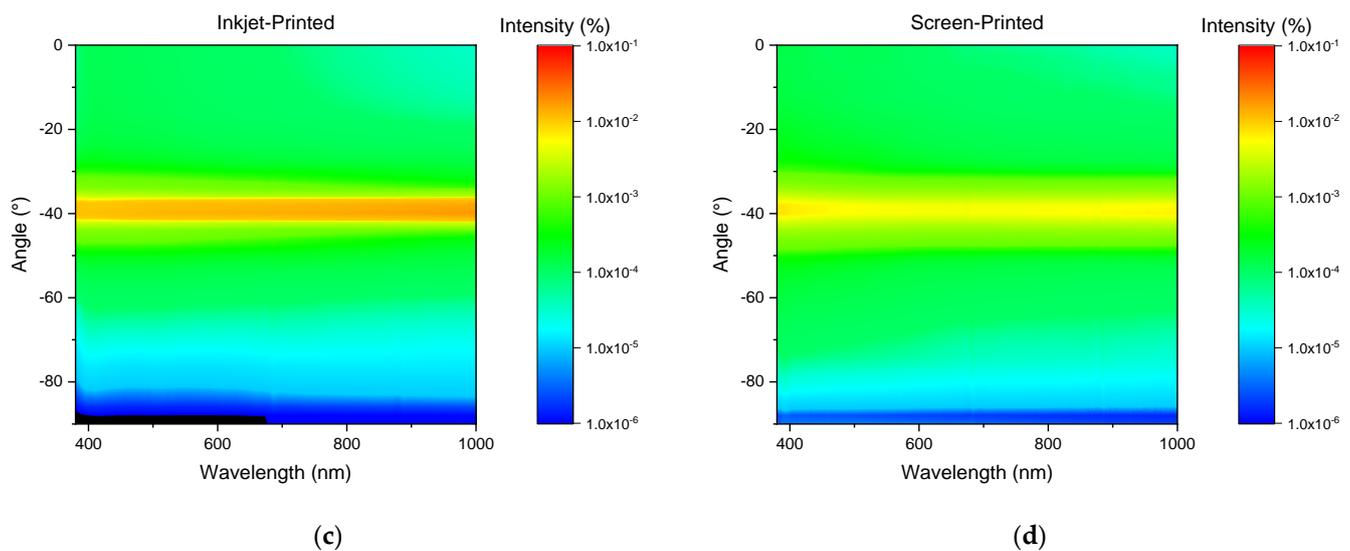
**Figure 5.** Angle-resolved reflection spectra for an uncoated glass sample (a) and for grey-coloured front glass samples, coated by the three different technologies: sol-gel-coating (b), inkjet-printing (c) and screen-printing (d). The lowering of the reflection maximum and the broadening of the overall reflection is clearly visible for all coatings, compared to the bare glass. (angle of incidence:  $40^\circ$ ).
