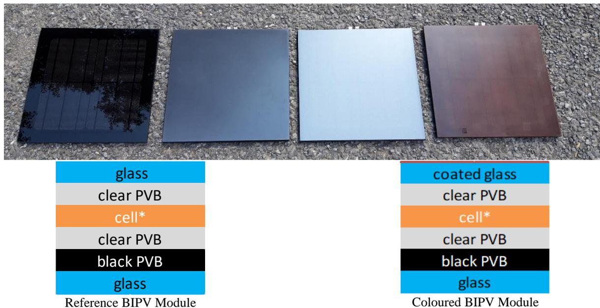
**Figure 2.** (Top): picture of test glass/glass photovoltaic modules (40 cm × 40 cm): from left to right: reference module, inkjet anthracite, screen-print grey, sol-gel terracotta. (Bottom): Scheme of reference and coloured BIPV modules.
