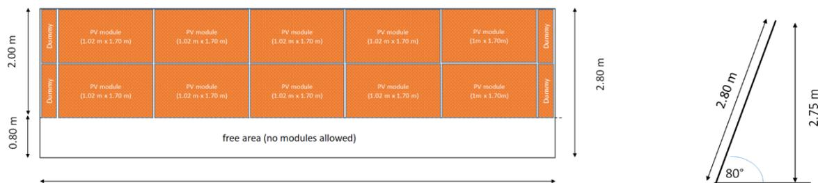
**Figure 11.** Design layout of the demonstrator facade in Mötz (Austria).
