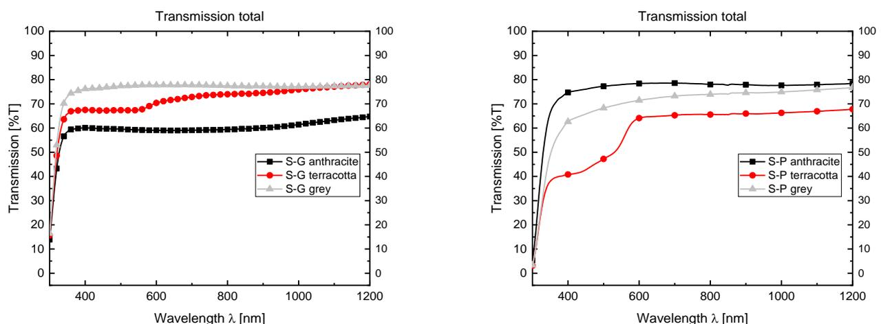
**Figure 6.** Transmission characteristics for coloured cover glasses coated by sol-gel (left) and screen-print (right) technologies.
