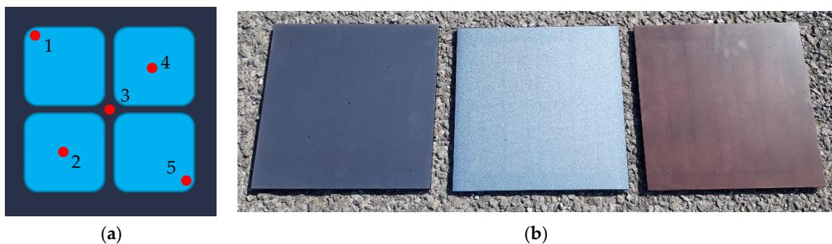
**Figure 9.** Hail test: (a) impact location; (b) picture of the test modules after the hail test: inkjet anthracite, screen-print grey, sol-gel terracotta (from left to right).
