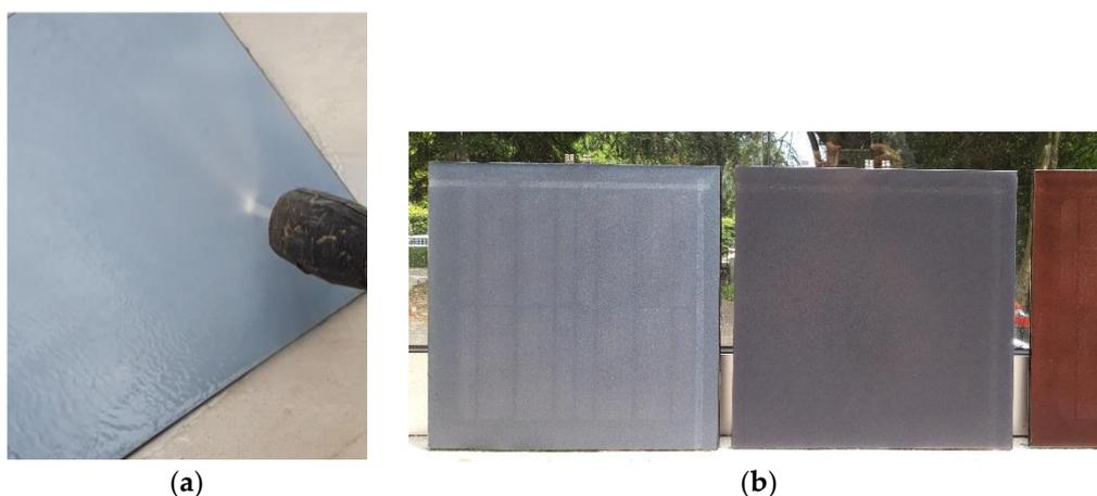
**Figure 10.** Pressure water-jetting test: (a) picture of the water jet; (b) picture of the test modules after the water jetting test: inkjet, anthracite, screen-print grey, sol-gel terracotta (from left to right).
