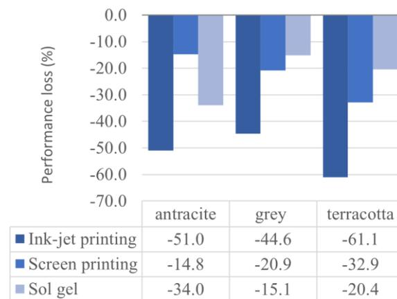
**Figure 7.** Estimated performance losses induced by each covered glass for a standard photovoltaic cell with respect to an uncoated glass, calculated as the ratio of the effective hemispherical transmittance of photon irradiance,  $\tau_e$ .
