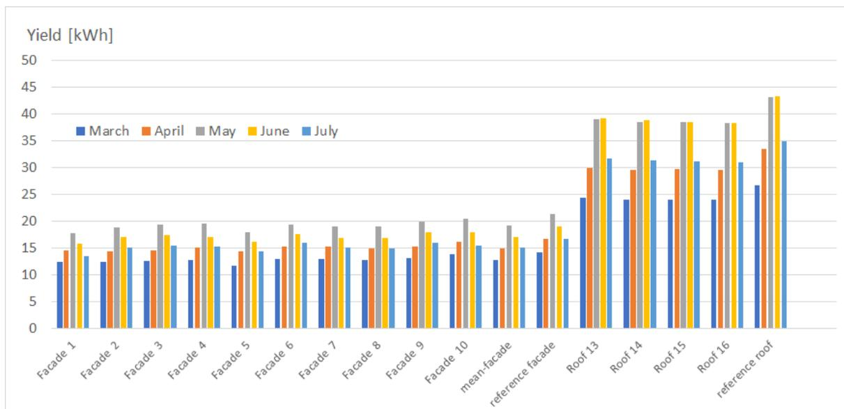
**Figure 13.** Performance data of the façade and roof modules of the test system in Mötz for the months from March 2021 to July 2021. The respective yield in kWh is shown for the reference modules, as well as for the grey-coloured modules coated by screen printing.
