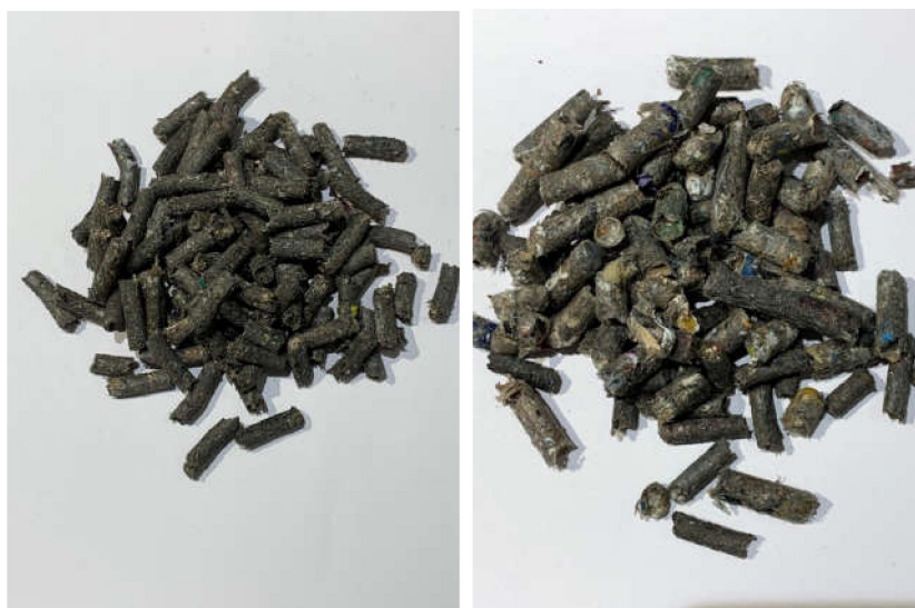
Figure 1. Typical 6 and 8 mm RDF Pellets (photo—J. Januszewski).
