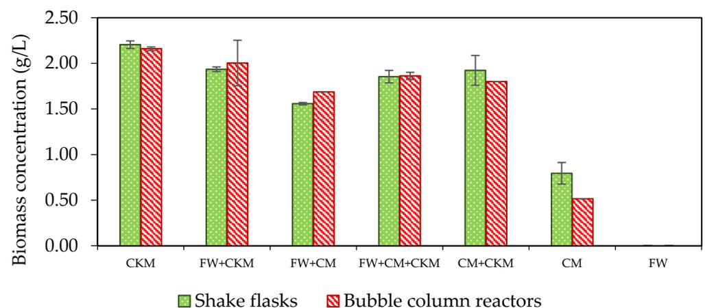
**Figure 1.** *A. oryzae* fungal biomass produced during cultivation in shake flask and in bubble column reactors.
