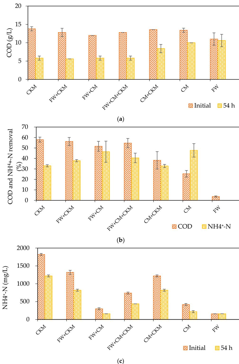
**Figure 4.** COD and ammonium content after cultivation of *A. oryzae* in VFA effluents derived in bubble column reactors: (a) COD content, (b) Ammonium content, (c) COD and Ammonium removal ratios (%).
