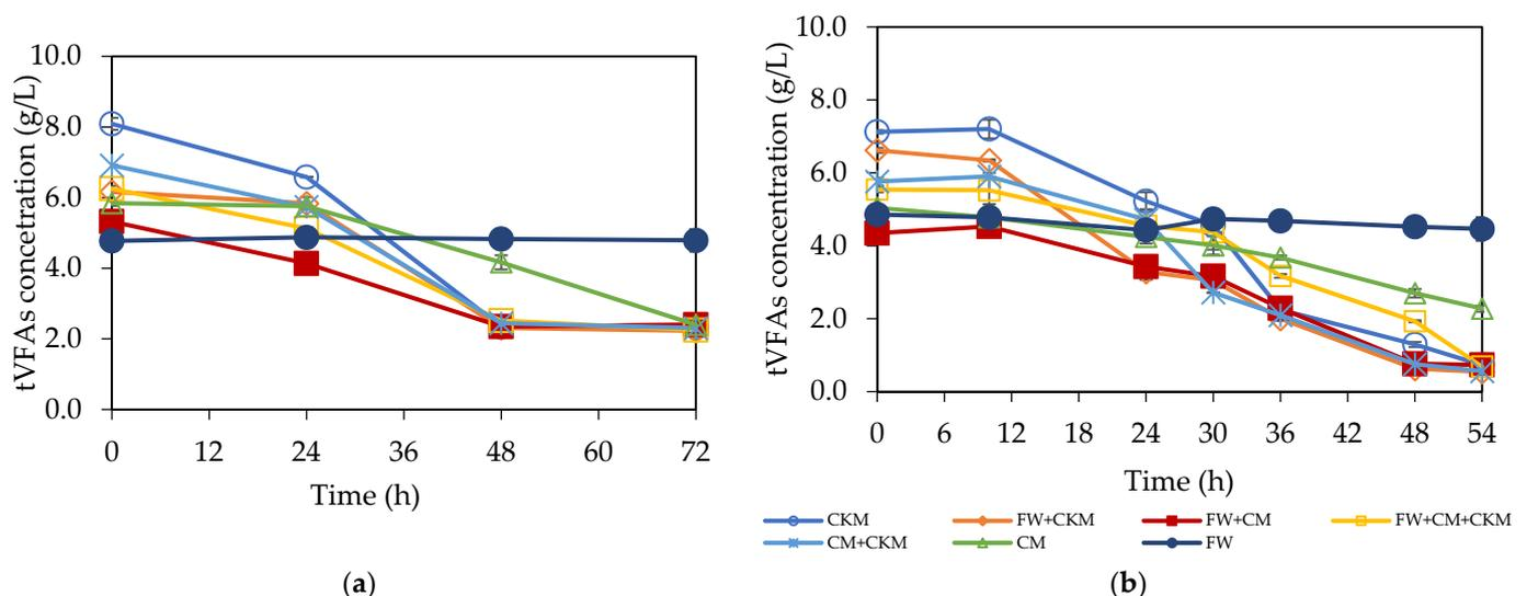
Figure 3. Total VFAs consumption profile by *A. oryzae* in VFAs effluent derived from cow manure, chicken manure and food waste (a) in shake flasks and (b) in bubble column reactor.
