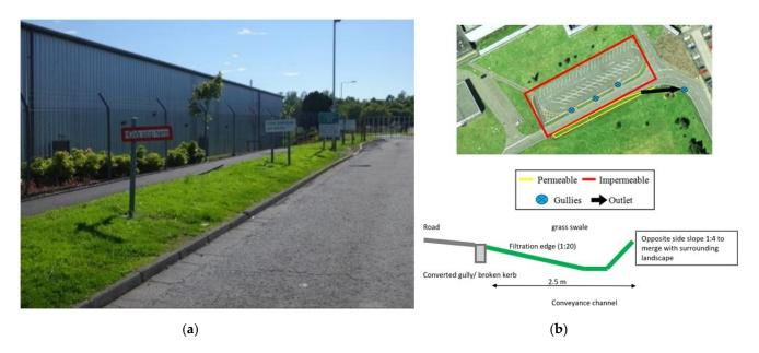
**Figure 15.** (**a**) Grass verge at Company B approach road, which could be converted to be a swale. (**b**) Technical schematic for the retrofit swale.
