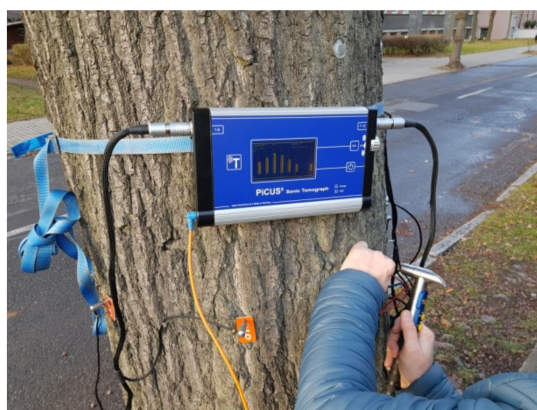
Figure 2. Measuring the geometry of the tree trunk using the PiCUS Calliper (M. Dudkiewicz, 2021).
