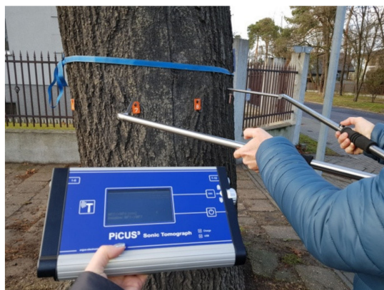
Figure 1. CT sonic scanner located on a tree trunk (M. Dudkiewicz, 2021).
