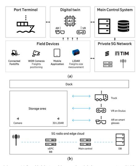
**Scheme 1.** (a) G-enabled devices of the control module for cargo operations. (b) 5G-enabled processes of the control module for cargo operations (Authors' elaboration).
