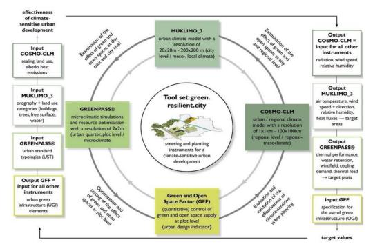
**Figure 14.** The multi-scale Green.Resilient.City toolset as steering, evaluation and optimisation investment at various climate and planning levels (ILAP/GRC project consortium).
