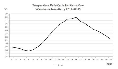
**Figure 4.** 2-m daily temperature cycle for the idealised summer day (19 July 2014) in COSMO-CLM used as input parameter for the two other climate simulation tools (AIT).
