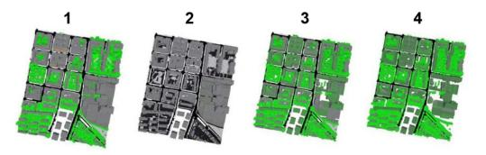
**Figure 7.** GREENPASS scenarios and simulation models ground plan: status quo (1), worst case (2), moderate case (3), and maximum case (4) (Green4Cities/GREENPASS, 2018).
