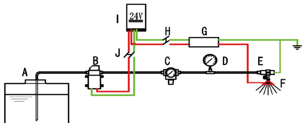
**Figure 2.** Schematic diagram of electrostatic spraying system: (A) tank; (B) diaphragm pump; (C) pressure gauge; (D) pressure regulator; (E) electrode; (F) fan nozzles; (G) electrostatic generator; (H) switch of electrostatic generator; (I) DC power supply; (J) switch of diaphragm pump.
