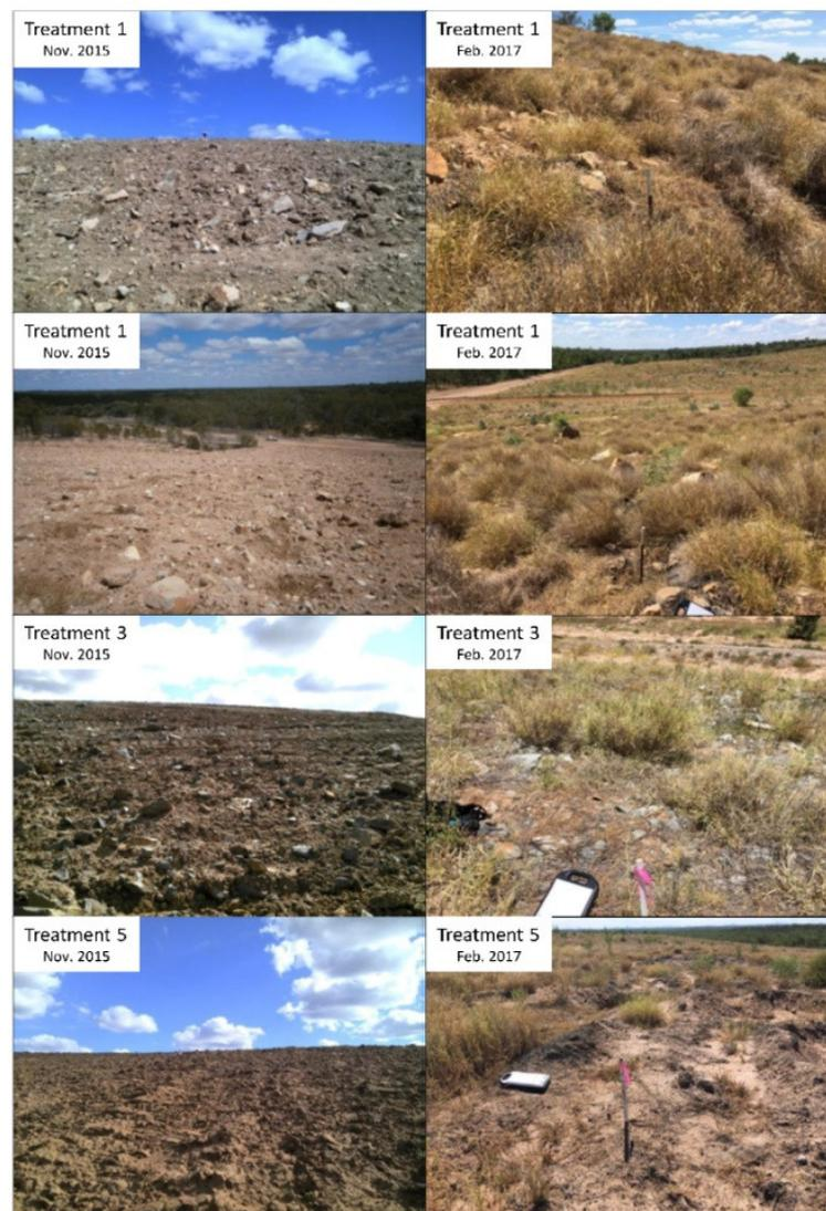
**Figure 4.** The experimental trials at German Creek East in November 2015 and February 2017. The selected spoil treatments are full rock mulch at 500 mm (Treatment 1), Gypsum + 100 mm rock mulch (Treatment 3) and Topsoil, rip, seed, and gypsum (Treatment 3).
