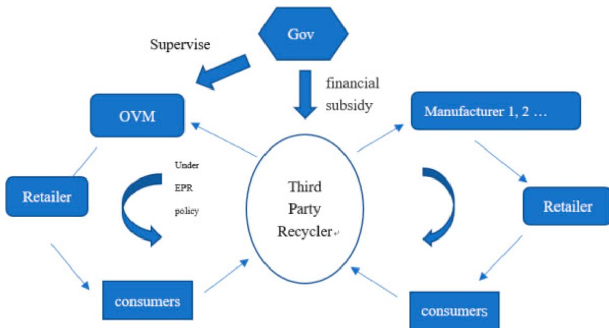
**Figure 1.** Dual-cycle ELV recycling and remanufacturing system.
