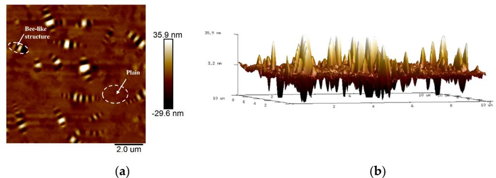
**Figure 4.** AFM figures of asphalt: (a) two-dimensional height of asphalt; (b) three-dimensional height of asphalt.
