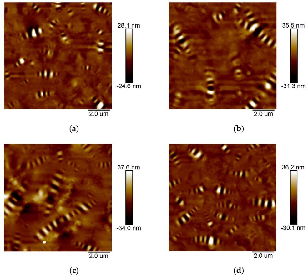
**Figure 9.** Two-dimensional nano-morphology AFM figures of asphalt with different eggshell waste contents: (a) neat asphalt, (b) 5% ESP, (c) 10% ESP, (d) 15% ESP.
