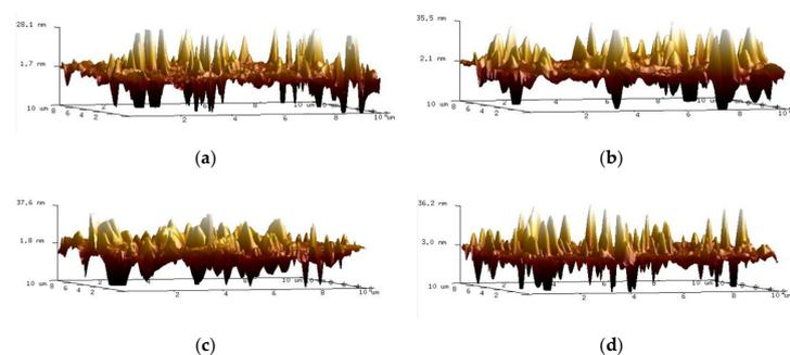
**Figure 10.** Three-dimensional nano-morphology AFM figures of asphalt with different eggshell waste contents: (a) neat asphalt, (b) 5% ESP, (c) 10% ESP, (d) 15% ESP.
