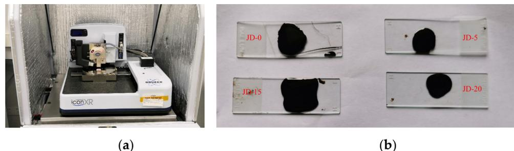
**Figure 3.** AFM test: (a) AFM instrument; (b) asphalt samples.
