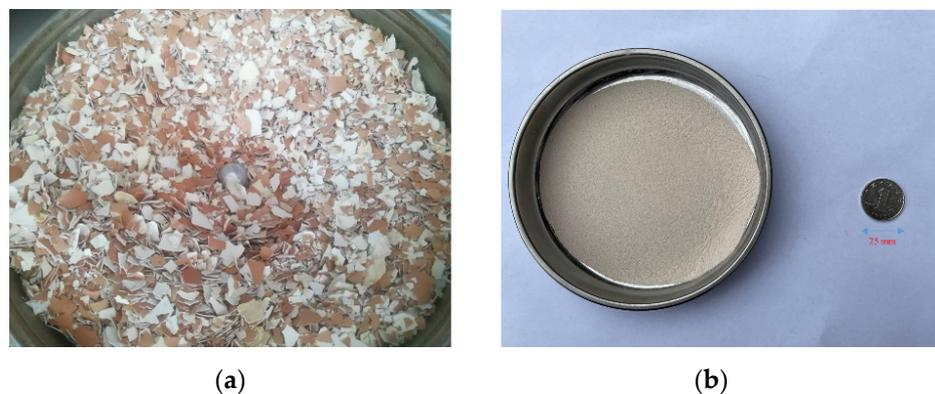
**Figure 1.** Appearance of eggshell material: (a) crushed eggshell; (b) eggshell powder.
