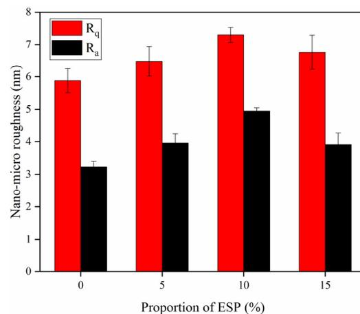
**Figure 11.** Nano-micro roughness of asphalt with different contents of eggshell waste.
