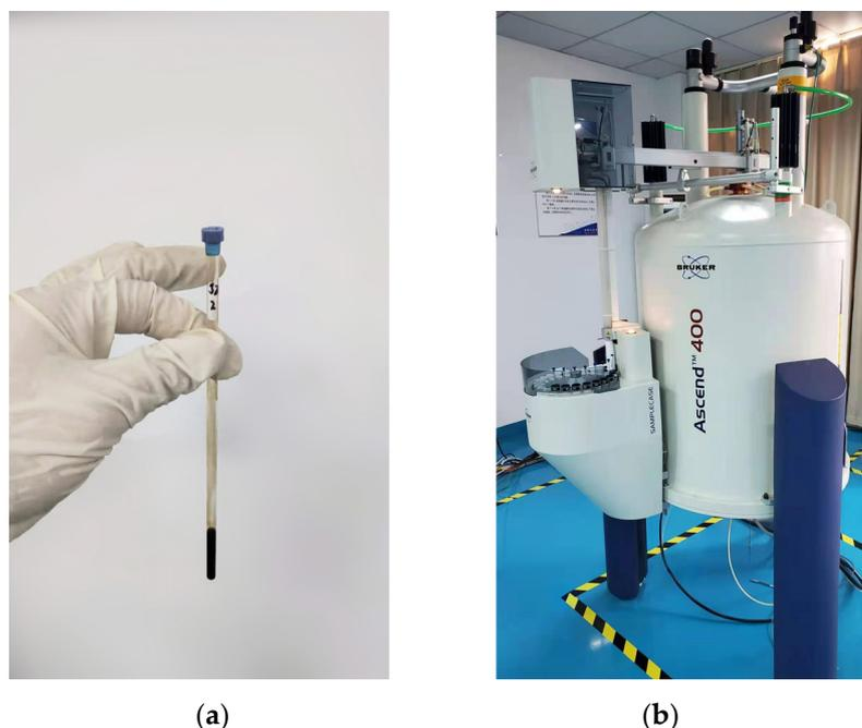
**Figure 2.**  $^1\text{H-NMR}$  test: (a) dissolve sample; (b) NMR equipment.
