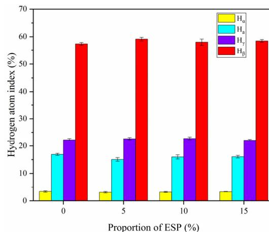
**Figure 7.** H-index distribution diagram of asphalt with different contents of eggshell waste.
