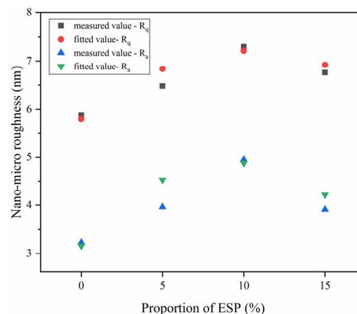
**Figure 12.** The fitting effect of the nano-micro indexes of asphalt at different contents of eggshell waste.
