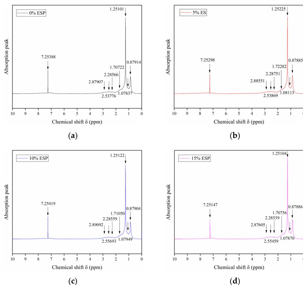
**Figure 6.** The  $^1\text{H}$ -NMR of asphalt with different contents of eggshell waste: (a) neat asphalt; (b) 5% ESP; (c) 10% ESP; (d) 15% ESP.
