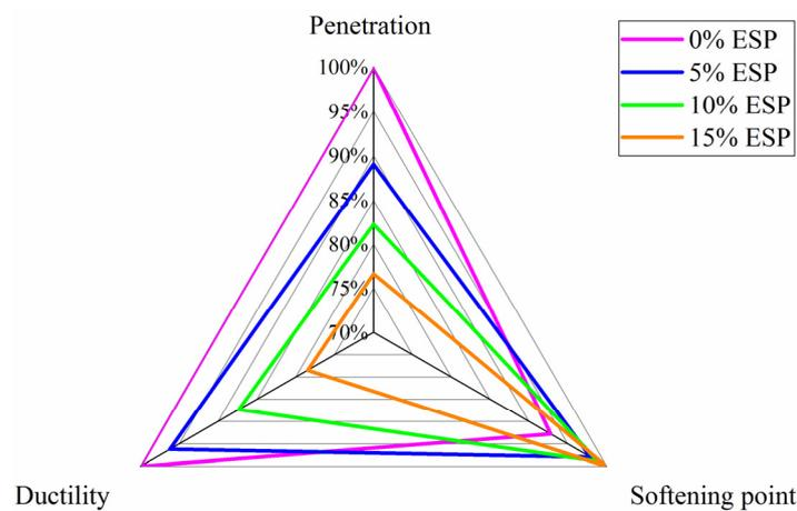
**Figure 5.** The hardness, thermal stability and ductility of asphalt with different contents of eggshell waste.
