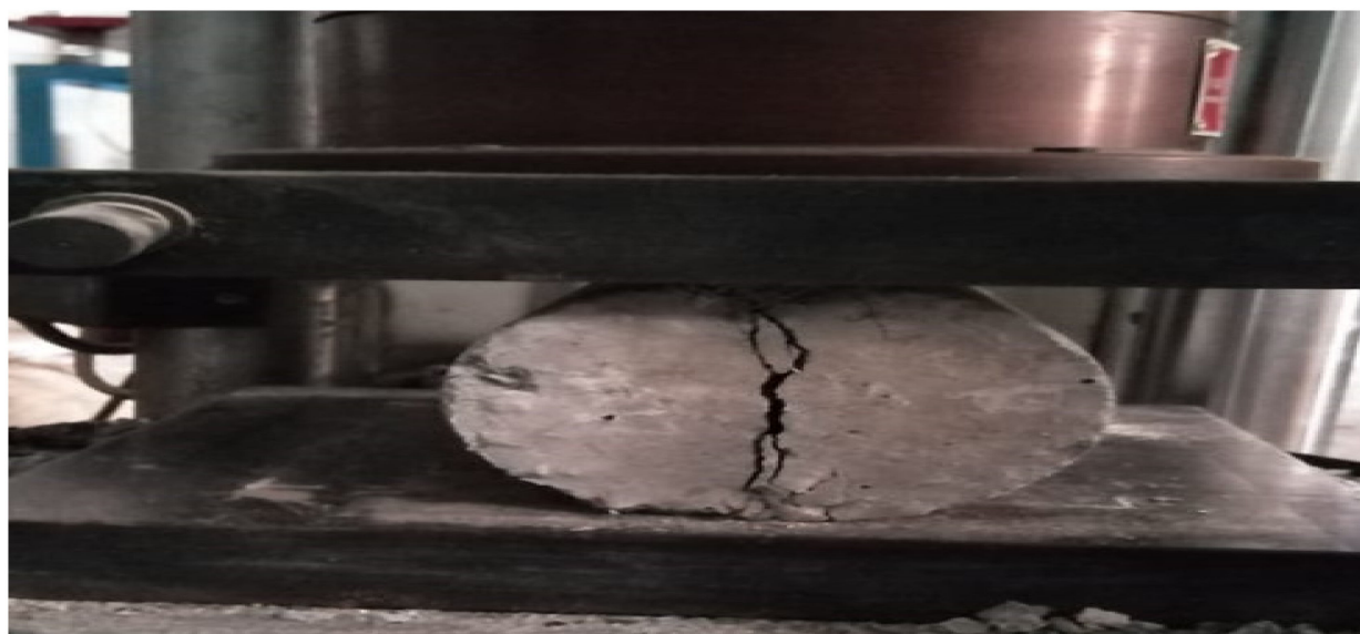
Figure 11. Split tensile strength setup.
