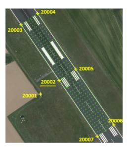
Figure 3. Basic (zero) geodetic net and GRID on the runway.
