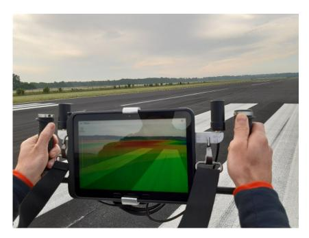
Figure 9. Display of surface deformations on the tablet.
