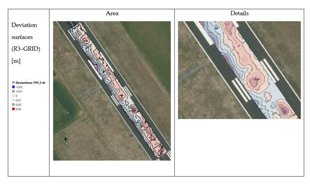
Figure 6. The result from the calculation of the R3 planes with the »QGIS« (Quantum GIS).
