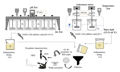
Figure 2. Experimental procedure for struvite precipitation in pH and temperature tests.
