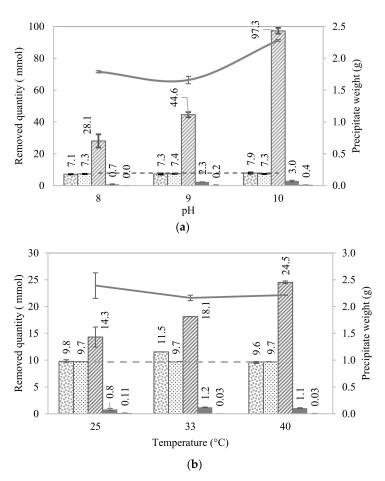
**Figure 3.** Removed quantities of Mg, P, N, Ca and K from the solution and recovered mass as a precipitate in pH (a) and *t* (b) tests. Symbols: Mg, P, M, Ca, Ca, K — precipitate mass, — maximum quantity (mmol) that can precipitate as struvite.
