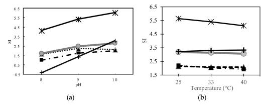
**Figure 4.** Saturation index (*SI*) calculated with Visual MINTEQ software for expected precipitates at (a) pH = 8, 9 and 10; (b) temperature = 25, 33 and 40 °C. Symbols: Struvite MgNH<sub>4</sub>PO<sub>4</sub>.6H<sub>2</sub>O, — Magnesite MgCO<sub>3</sub>, ··· · · Calcite CaCO<sub>3</sub>, — Farringtonite Mg<sub>3</sub>(PO<sub>4</sub>)<sub>2</sub>, — Amorphous calcium phosphate Ca<sub>3</sub>(PO<sub>4</sub>)<sub>2</sub>.
