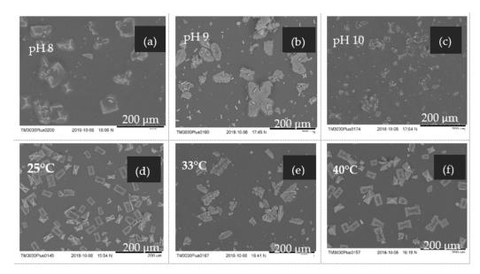
**Figure 6.** SEM images of precipitates obtained in pH-tests at T = 20 °C (**a**–**c**) and temperature tests at pH 9 (**d**–**f**) trials.
