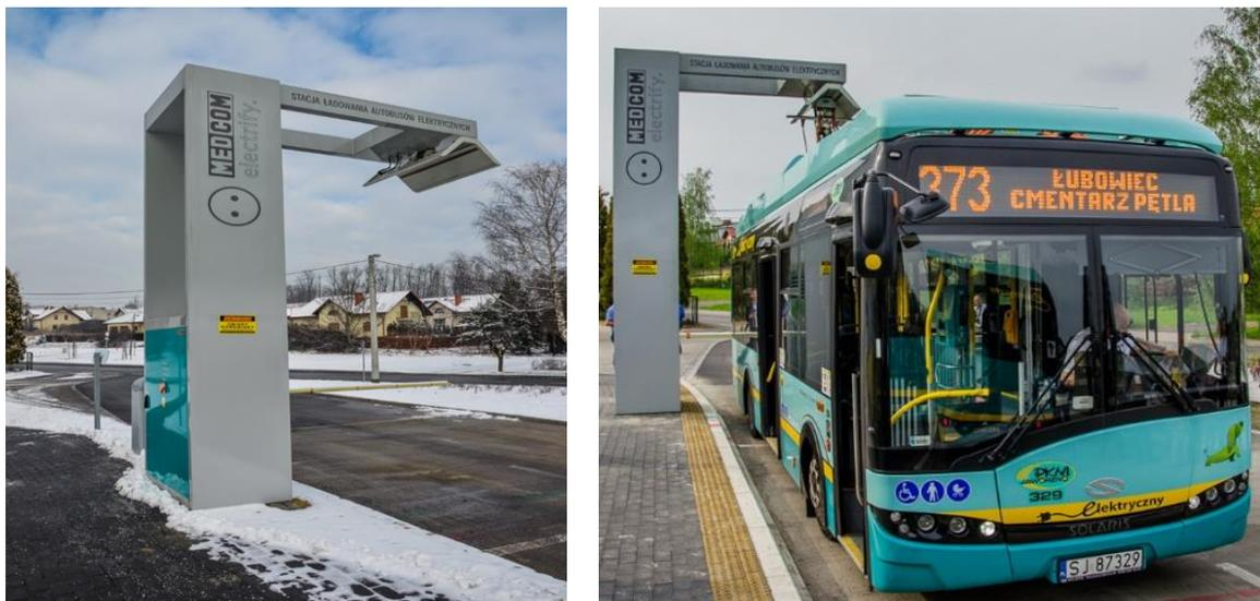
Figure 10. Pantograph charging solution in Szpital Pętla.
