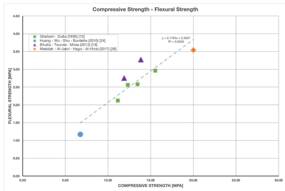
Figure 4. Relationship between compressive strength and flexural strength of porous concrete.
