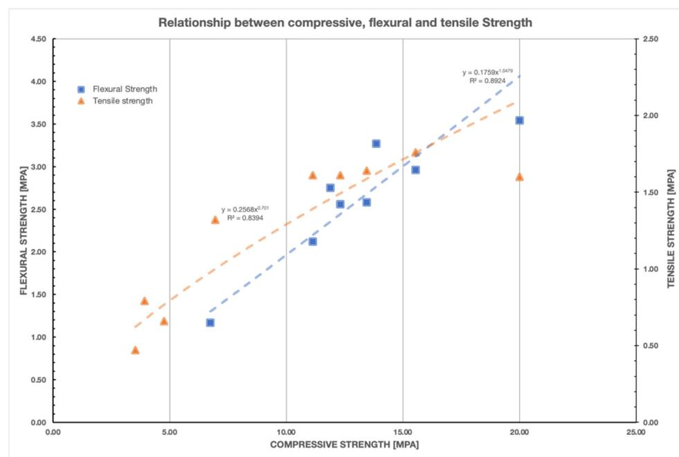
Figure 5. Relationship between compressive, tensile and flexural strength.
