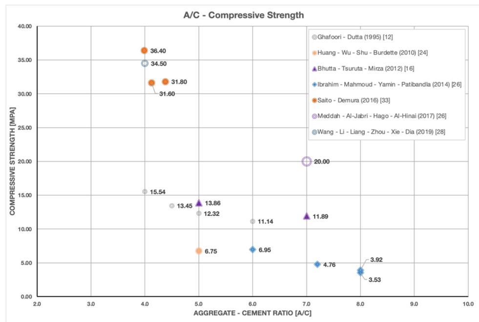
**Figure 2.** Relationship between aggregate–cement ratio and the compressive strength.
