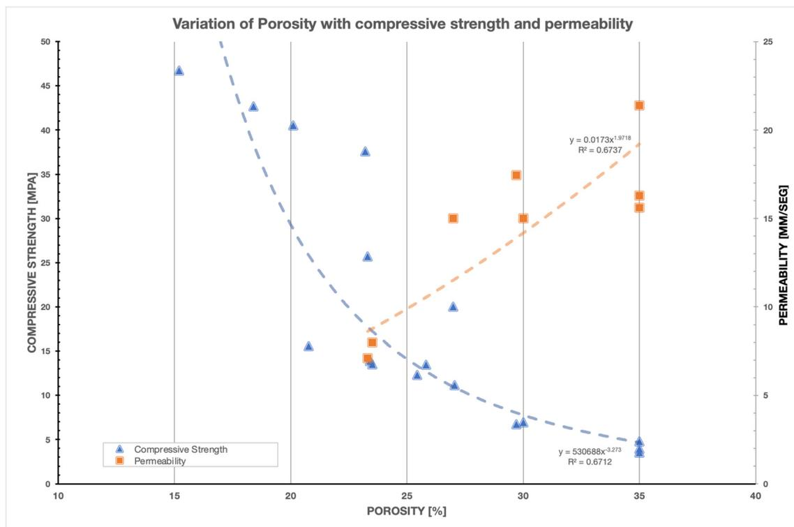
Figure 10. Estimated variation of porosity versus the results obtained for compressive strength and permeability.
