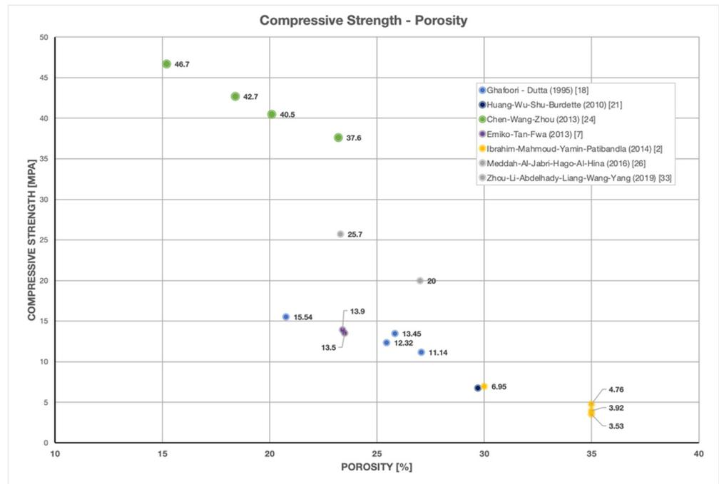
Figure 8. Relationship between porosity and compressive strength.
