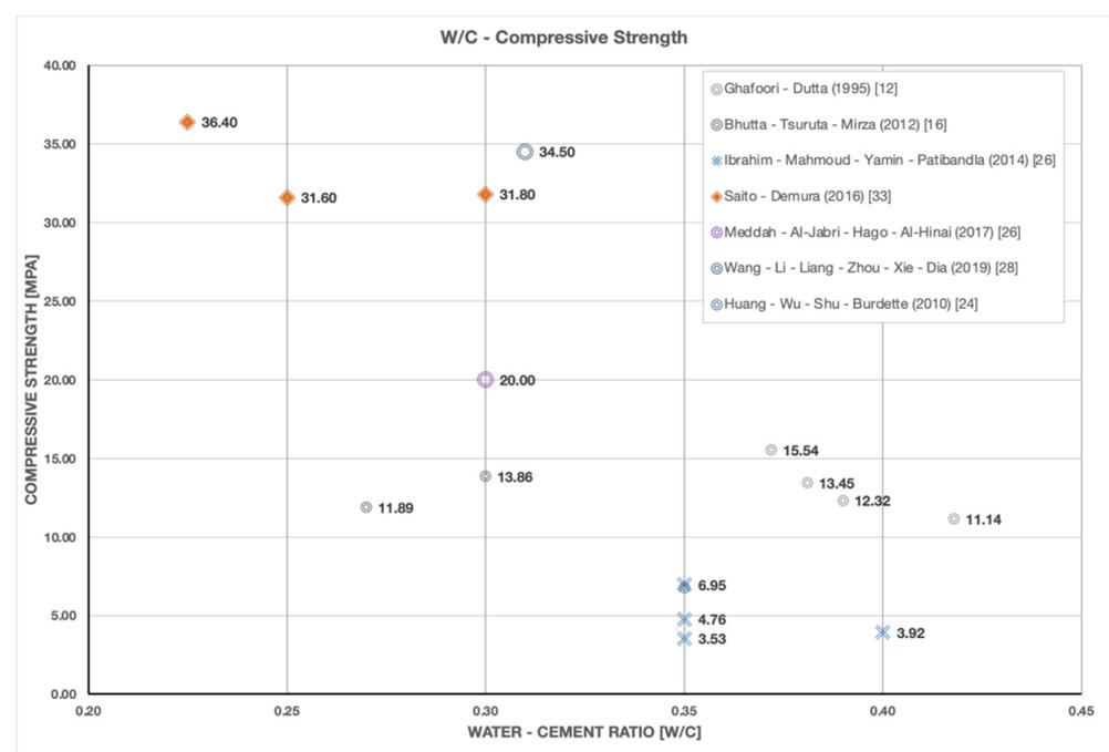
**Figure 1.** Relationship between water–cement and the compressive strength.
