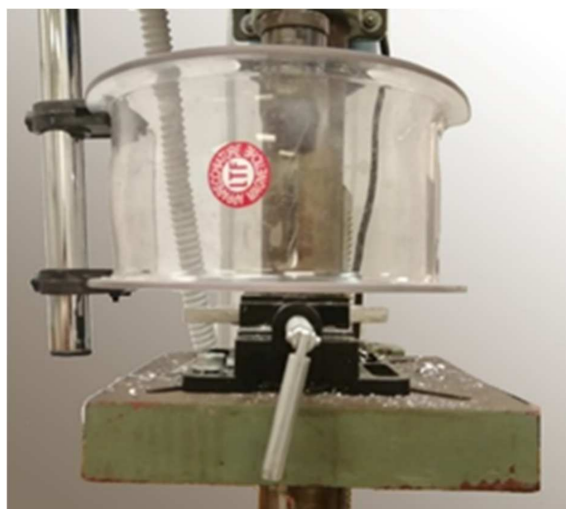
Figure 7. Installation of the protection screen on the drill press.
