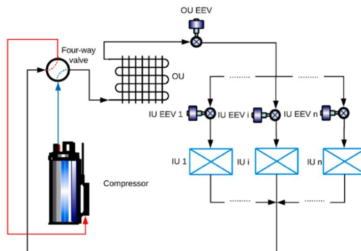
Figure 2. Simplified VRF diagram [5].
