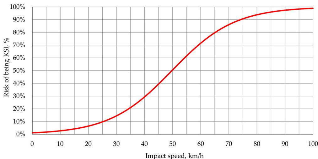
**Figure 1.** Risk of being killed or severely injured (KSI) in relation to impact speed, based on [5].
