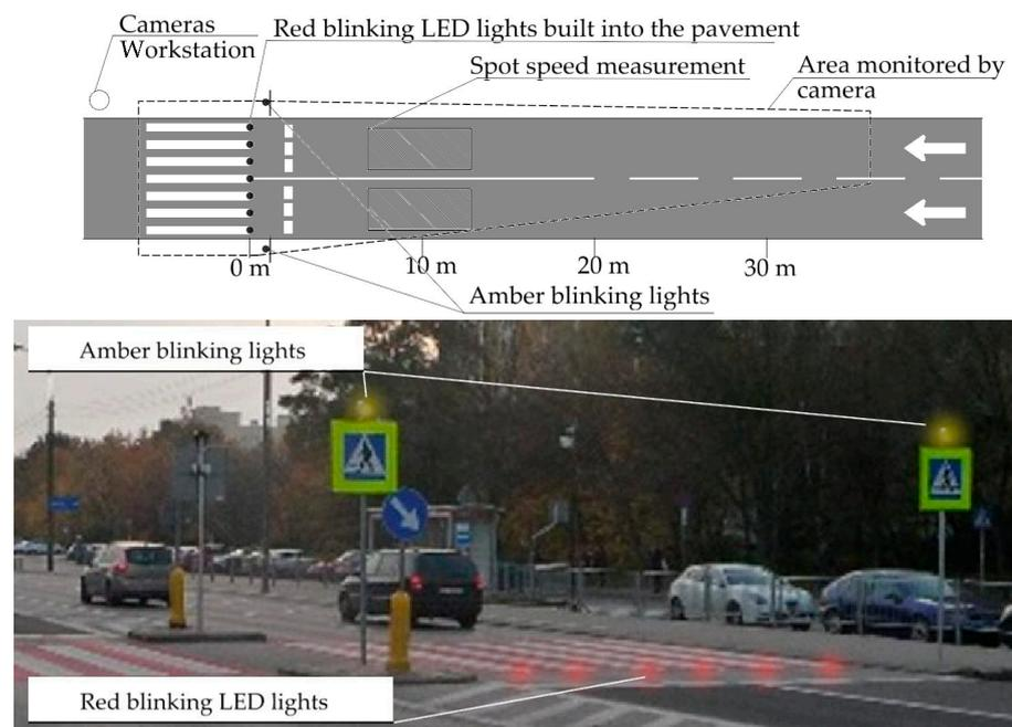
**Figure 3.** Typical layout and photograph of the implementation study test site.
