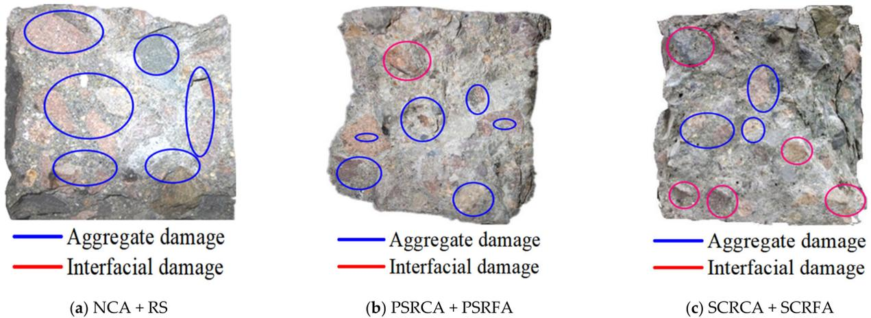
**Figure 10.** Fracture interface of concrete block.
