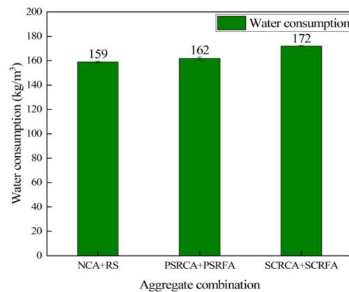
**Figure 8.** Water consumption of fully recycled concrete.
