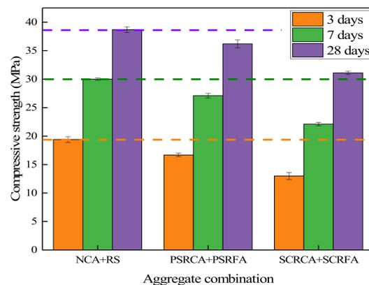
**Figure 9.** Compressive strength of concrete at different ages.
