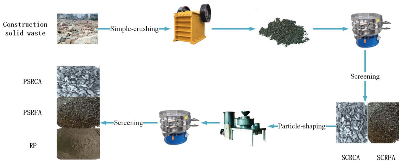
**Figure 1.** Flow chart of construction solid waste treatment.
