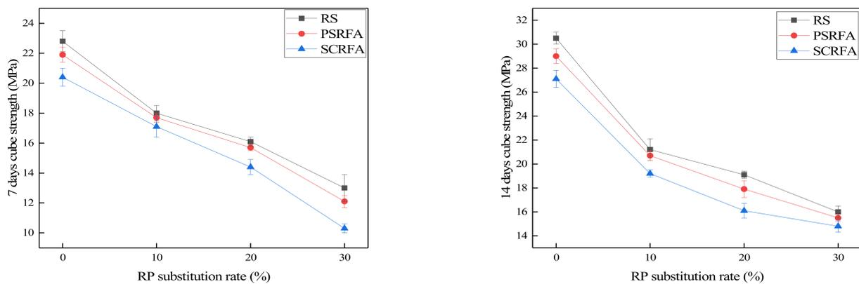
(a) 7d compressive strength of dry-mixed masonry mortar
