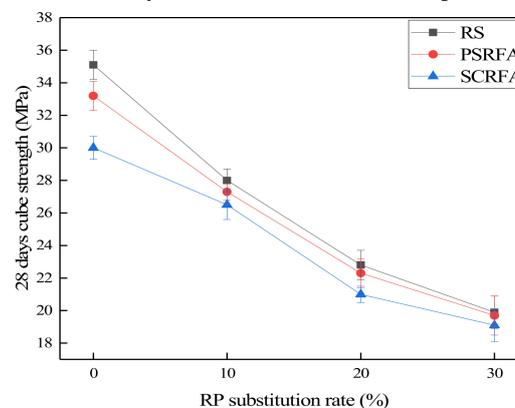
(c) 28 d compressive strength of dry-mixed masonry mortar
