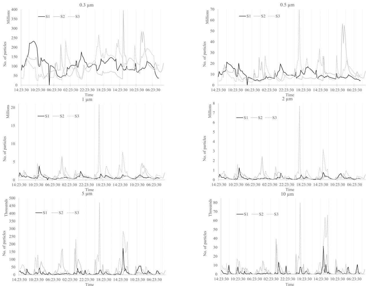
**Figure 2.** Results regarding the number of particulate matter measured in three different spots (S1—in the furthest point relative to the living room tilt-opened window; S2—near the living room tilt-opened window and S3—near the balcony’s tilt-opened window) and for six different dimensions (0.3; 0.5; 1; 2; 5 and 10  $\mu\text{m}$ ).
