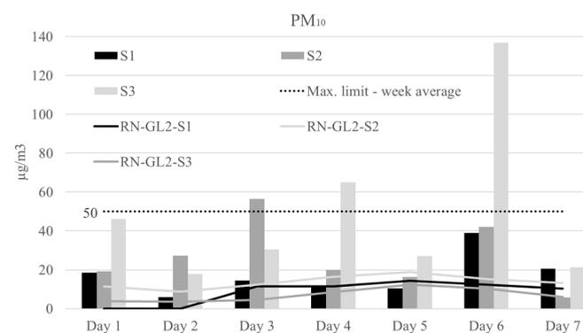
**Figure 5.** Daily mean values of  $PM_{10}$ , expressed in  $\mu\text{g}/\text{m}^3$ , registered in the three measurement spots (S1, S2 and S3), compared with the maximum admissible value according to the national legislation and the weekly mean values registered by the closest measuring station of the national measuring system (RN-GL2-S1, RN-GL2-S2 and RN-GL2-S3) during the same time as this study measurement period.
