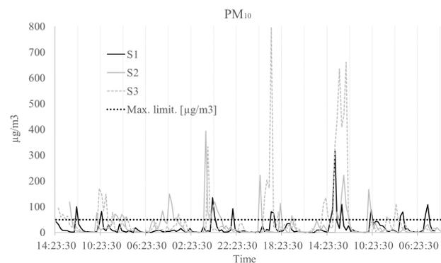
**Figure 4.** Hourly mean values of  $PM_{10}$ , expressed in  $\mu\text{g}/\text{m}^3$ , registered in the three measurement spots (S1, S2 and S3), compared with the maximum admissible value according to the national legislation.
