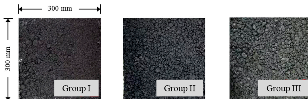
Figure 2. The fabricated samples used for the polishing test.
