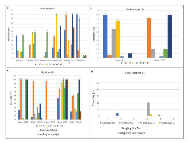
**Figure 2.** Toxicity of airport runoff water samples towards *Thamnocephalus platyurus* determined by the Thamnotoxkit F<sup>TM</sup> test. (**a**). Small Airport PL; (**b**). Medium Airport PL; (**c**). Big Airport PL; (**d**). Large Airport UK.
