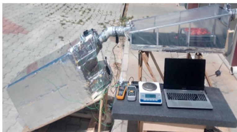
Figure 17. Experimental setup of the QPSAC integrated with a GHD, adapted with permission from [104].
