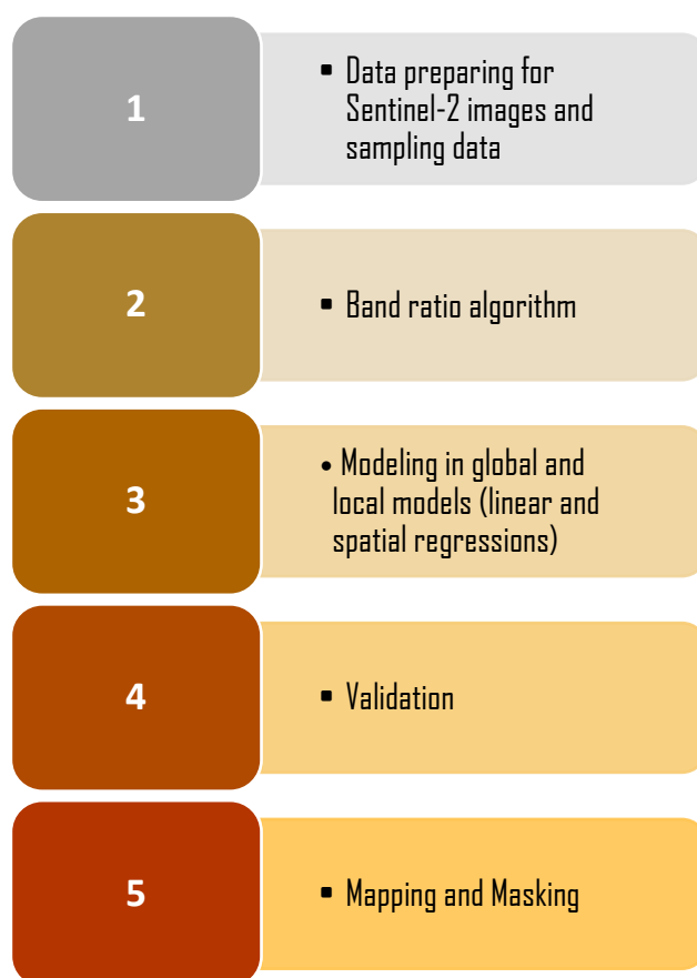
Figure 2. Processes of the water quality mapping system, including (1) data preparing for Sentinel-2 images and sampling data; (2) band ratio algorithm, i.e., blue-green, green-red, the red-NIR (near infrared) band ratios and the three-band approaches; (3) global and local models of mapping, e.g., linear and spatial regressions in Equation 9 and Equation 10; (4) validation, (5) mapping, and masking based on NDWI (normalized difference water index).
