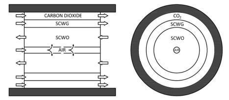
Figure 2. Internal design of the supercritical water gasification and oxidation reactor.
