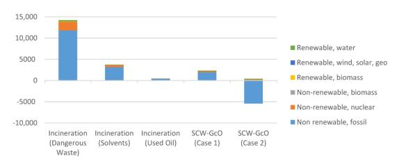
**Figure 8.** Comparison of the primary energy consumption between the incineration processes and SCW-GcO (working phase).
