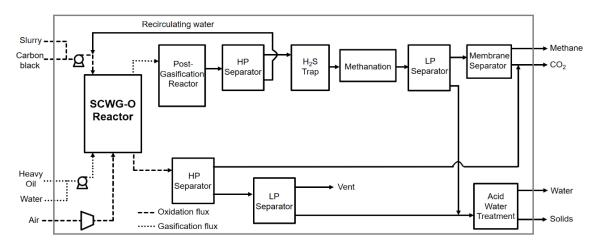
Figure 3. Life cycle flowchart of the overall system.
