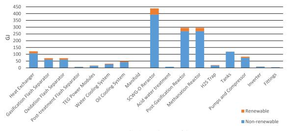
Figure 4. Primary energy for the production of the components.
