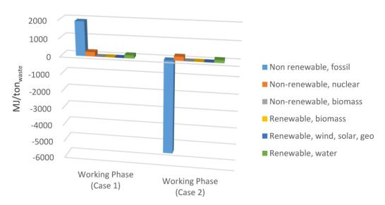
Figure 6. Comparison of the primary energy consumption for Case 1 and Case 2 (working phase).
