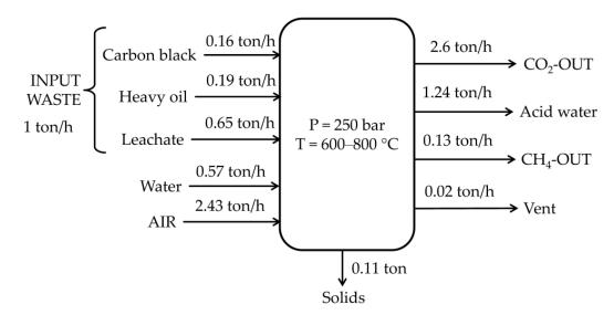
Figure 5. Mass balance of the SCW-GcO system.
