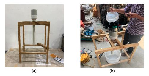
Figure 5. Equipment and progress for the permeability test. (a) device for test; (b) test process.
