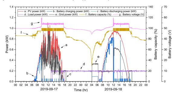
Figure 7. Performance characteristics of BESS prototype with balcony PV based on mode 4 (17–18 September 2019).
