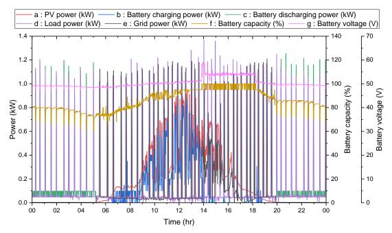
Figure 8. Performance characteristics of BESS prototype with balcony PV applied the air conditioner's load (7 July 2019).
