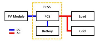
Figure 1. Schematic diagram of battery energy storage system (BESS) with photovoltaic system (PV).
