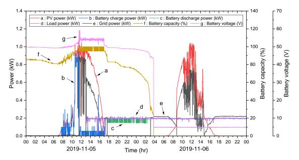
Figure 6. Performance characteristics of BESS prototype with balcony PV based on mode 3 (5–6 November 2019).
