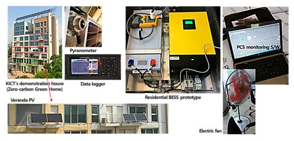
Figure 2. Photographs of the building and experiment apparatus.
