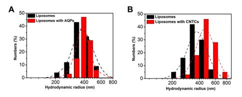
Supplementary Fig.4. The change in particle size of liposomes after insertion into the water channel. The change in the particle size of liposomes after insertion of AQPs (Fig.7A); the change in the size of liposomes after insertion of CNTC (Fig.7B). It can be seen from the figure that the particle size distribution of the vesicles is almost unchanged after being inserted into the water channel, that is, the insertion of the water channel has no obvious effect on the vesicles.
