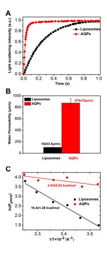
Supplementary Fig.6. Light scattering curves of DOPC and AQPs (Figure A); water permeability of DOPC and AQPs calculated based on light scattering curves (Figure B); Arrhenius diagram showing the water permeability of DOPC liposomes and
