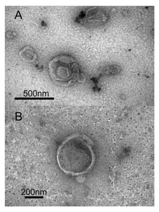
Supplementary Fig.7. Liposomes were stained with phosphotungstic acid (2%) and morphologically characterized by TEM.As shown in the figure, the liposomes are approximately round with a particle size distribution around 400 nm.
