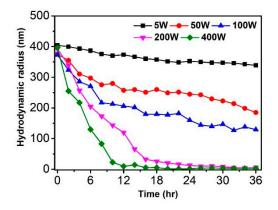
Supplementary Fig.1. The relationship between the length of CNTC and time under different ultrasonic power. It can be seen from the figure that under 200W power, the length of CNTC has a linear decreasing relationship with time.
