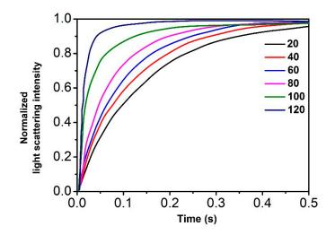
Supplementary Fig.5. Light scattering curve of CNTC under different osmotic pressure gradient.
