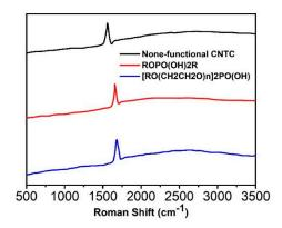
Supplementary Fig.2. Raman spectrum (black curve) of the unsuccessfully functionalized CNTC. Raman spectrum (red curve) of the sample after functionalization of CNTC with monolauryl phosphate as the active agent. Raman spectrum (blue curve) of the sample after functionalized CNTC with alcohol ether
