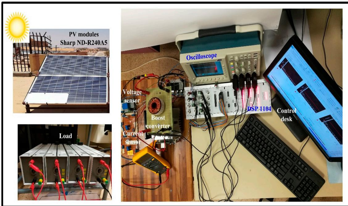
Figure 11. The PV system experimental setup.
