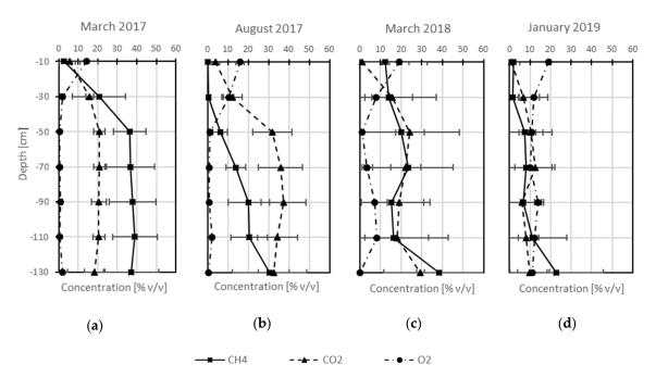
**Figure 3.** Biowindows soil gas composition of CH<sub>4</sub>, CO<sub>2</sub> and O<sub>2</sub>: (**a**) March 2017; (**b**) August 2017; (**c**) March 2018; (**d**) January 2019.
