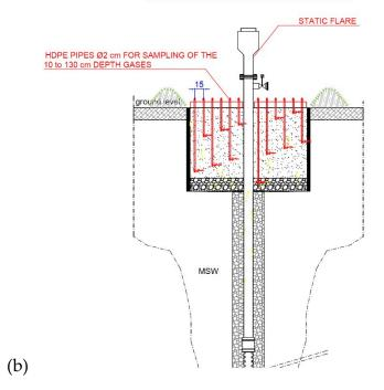
Figure 1. Biofilter (a) and Biowindow (b) sections (non-scale scheme).
