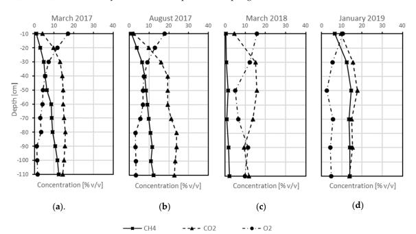
resulted 19.2  $\pm$  10.2 Nl/m<sup>2</sup>h. Figure 2 shows the profiles at different depths of concentration of CH<sub>4</sub>, CO<sub>2</sub> and O<sub>2</sub> in the four days of volatile compounds sampling in the biofilter.
