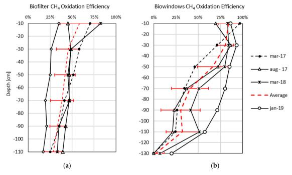
Figure 4. CH<sub>4</sub> oxidation efficiency: (a) biofilter; (b) biowindows.
