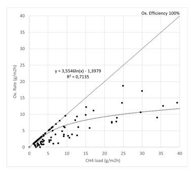
Figure 5. Logarithmic trend between CH<sub>4</sub> load and Oxidation efficiency in the biofilter.
