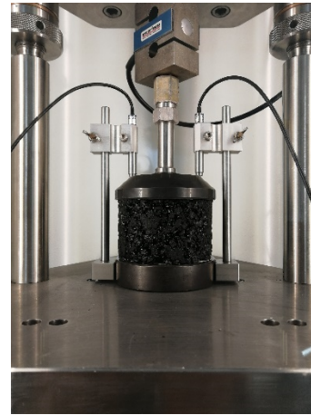
(b) The test piece in creep test
