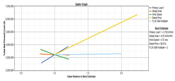
Figure 20. Spider graph presenting the effects of an O&M cost increase (two-fold) in total NPC.
