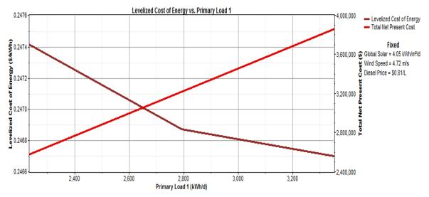
Figure 21. Line graph showing the characteristics of COE vs. NPC when the solar radiation is 4.05 kWh/m<sup>2</sup>/d.
