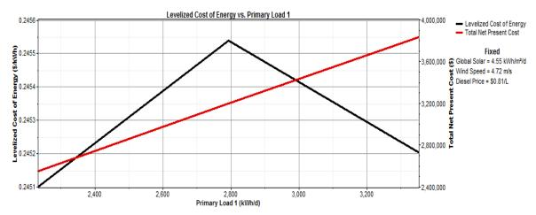
Figure 15. Line graph showing the characteristics of COE vs. NPC when the diesel price is \$0.81/L.
