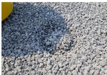
**Figure 8.** Footprint left by the ring-shaped foot of the SSG.
