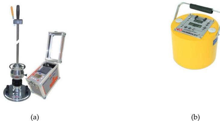
**Figure 2.** Devices for modulus evaluation: (a) light weight deflectometer (LWD) [24]; (b) soil stiffness gauge (SSG) [25].
