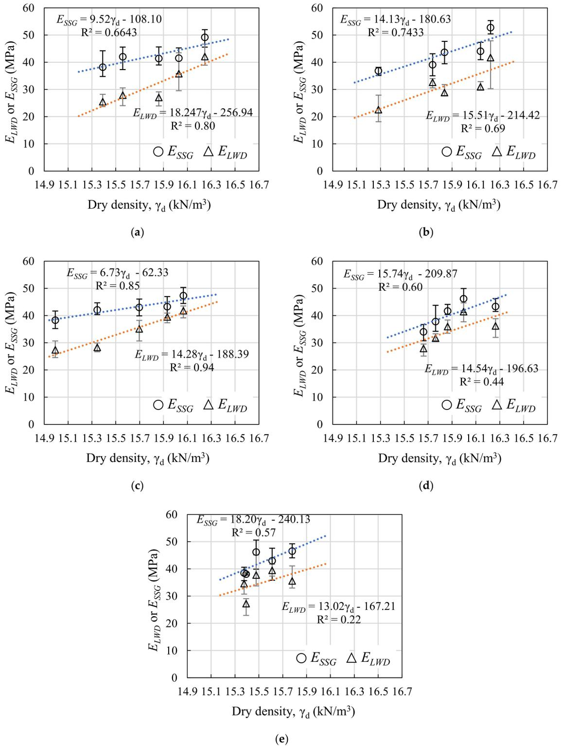
**Figure 10.** Relationship between dry density ( $\gamma_d$ ) and modulus ( $E_{LWD}$ ,  $E_{SSG}$ ): (a) D40; (b) D40 + D25; (c) D25; (d) D25 + D13; (e) D13. Note: the symbol and error bar represent the mean value, and the maximum and minimum values of the measurements, respectively.
