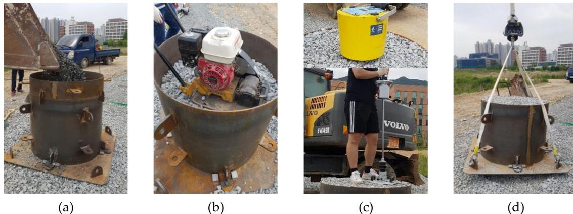
Figure 6. Soil chamber and modulus evaluation test procedure: (a) pouring test material into the mold; (b) compaction with vibratory plate compactor; (c) modulus evaluation with LWD and SSG; (d) weight measurement using hoist scale.
