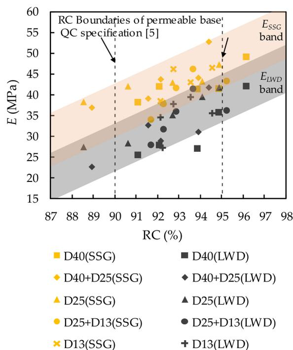
**Figure 11.** Relationship between relative compaction (RC) and modulus ( $E_{LWD}$ ,  $E_{SSG}$ ).
