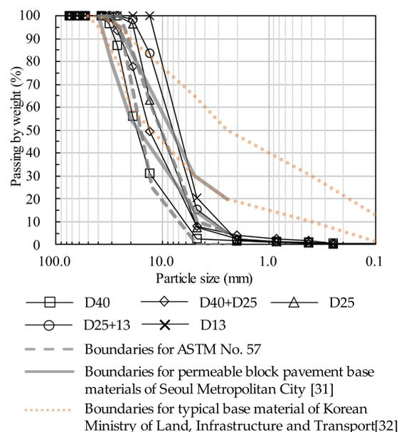
**Figure 4.** Particle size distribution of test materials and specifications (modified from Choi et al. [6]). Note: The particle size distributions of the test materials were obtained based on KS F 2502 [27].
