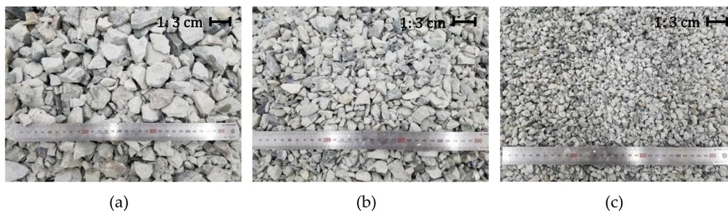
**Figure 3.** Air-dried open-graded aggregates (OGA) used for the test. The maximum particle sizes are: (a) 40 mm (D40); (b) 25 mm (D25); (c) 13 mm (D13) (modified from Choi et al. [6]).
