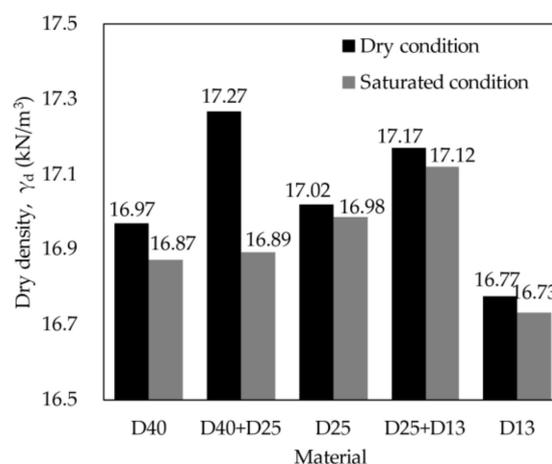
**Figure 9.** Results of vibratory hammer compaction tests. Note: The test was performed twice for each water content condition with each test material; Plotted values are mean values; The difference of the two test results agreed to within 2%, except for D40, which was 3%.
