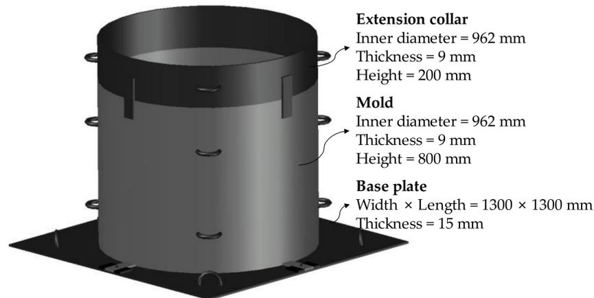
Figure 5. Schematic representation of the developed soil chamber.
