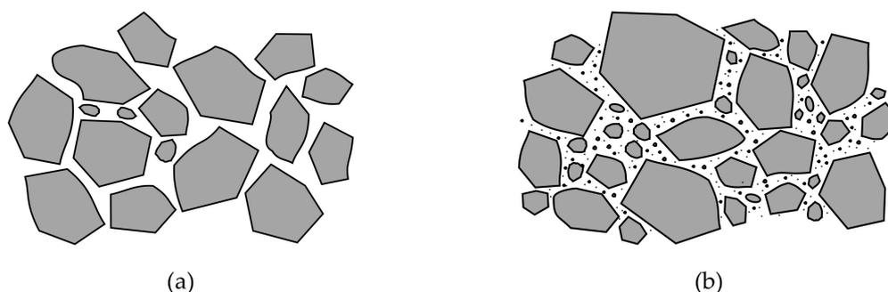
**Figure 1.** Conceptual illustration of pavement base materials [6]: (a) open-graded aggregates (OGAs); (b) dense-graded aggregates.
