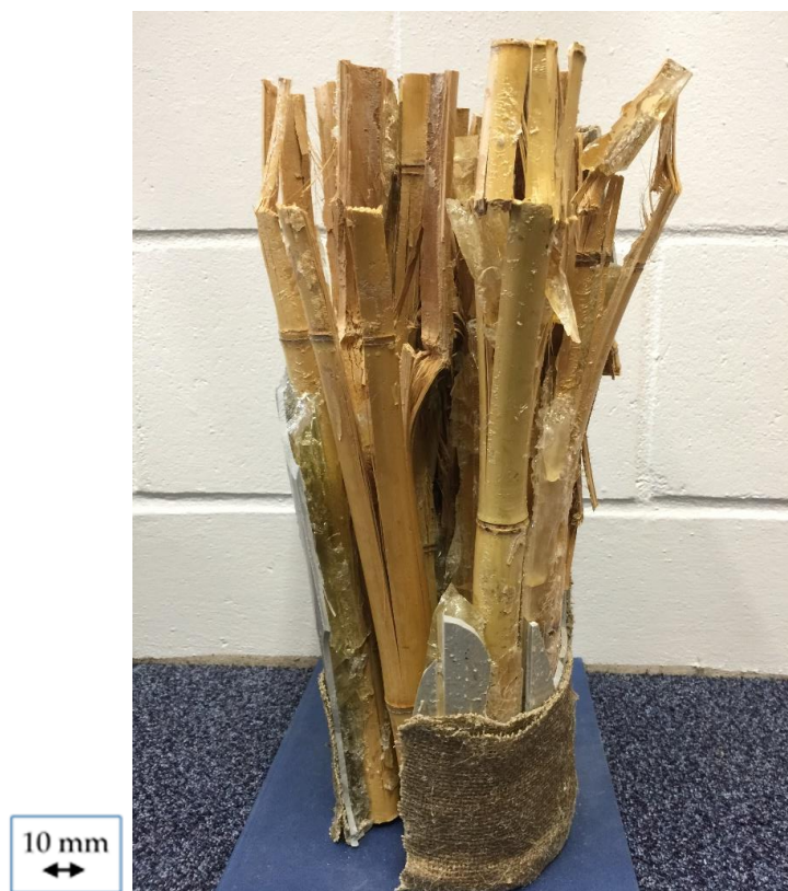
Figure 9. Failure mode of FCB-EXP-I specimen.
