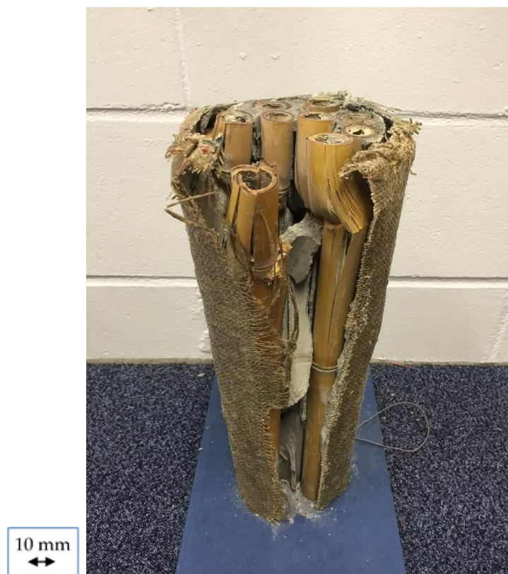
Figure 7. Failure mode of FCB- cementitious grout (GRT)-H specimen.
