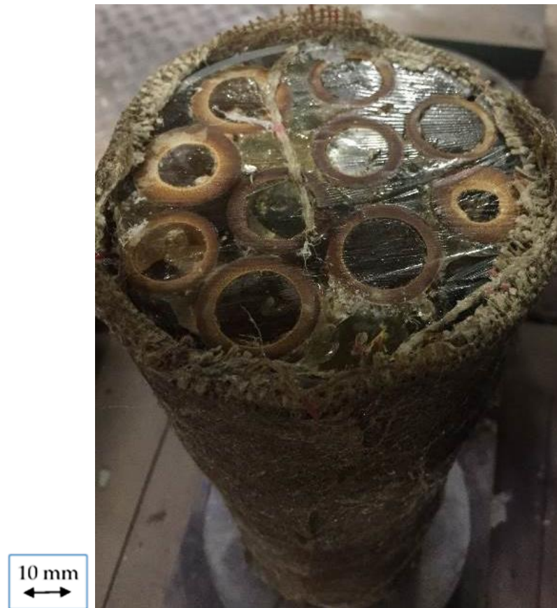
Figure 1. Cross-section of full culm bamboo composite (FCB)-epoxy matrix (EPX)-improved polyvinyl chloride (PVC) jacket (I) specimen before testing.
